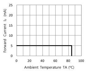
Fig. 2 FORWARD CURRENT VS. DERATING CURVE
