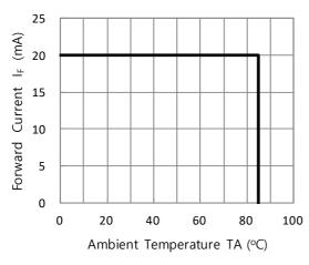
Fig. 2 FORWARD CURRENT VS. DERATING CURVE
