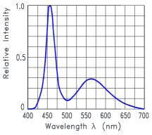
Fig.1 Relative Intensity VS. Wavelength
