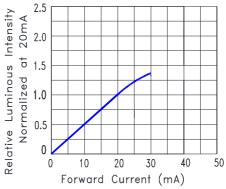
Fig.4 Relative Luminous Intensity vs. Forward Current
