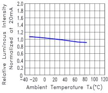
Fig.5 Relative Luminous Intensity VS. Ambient Temperature
