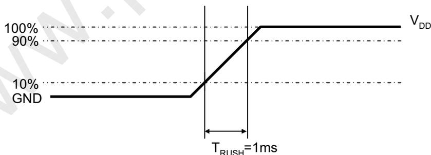
Rush Current  $I_{RUSH}$  can be measured when  $T_{RUSH}$  is 1ms.
