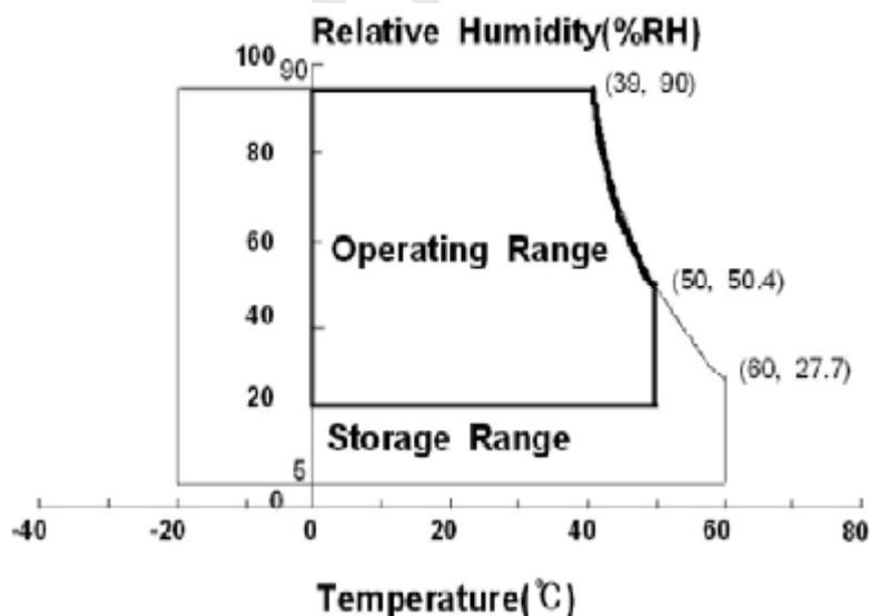
Fig. Temperature and Relative humidity range
