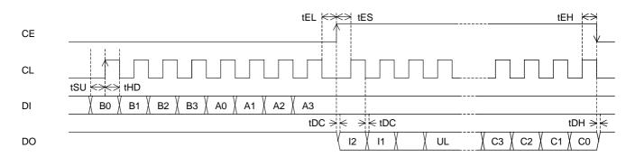
(Note) DO pin is an Nch open drain pin, so that the data varying time (tDC and tDH) differs depending on the pull-up resistance and substrate capacity.
