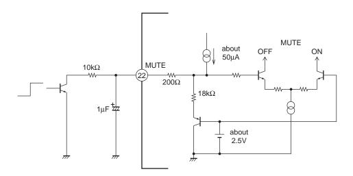
Fig2 Mute equivalent circuit
