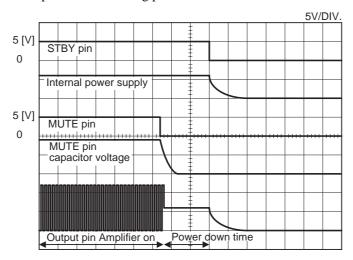
Turn-off time: the time between the point the MUTE pin is set low and the point the STBY pin is set low.
