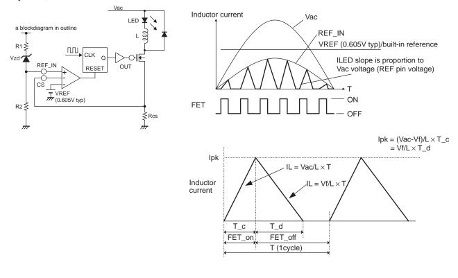
Given that the period when current flows into coil is
