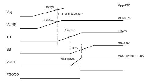
\* Starts charging the TD at the trigger point of either VIN > 9V(typ) or VLIN5 > 4.5V(typ), whichever is later.
