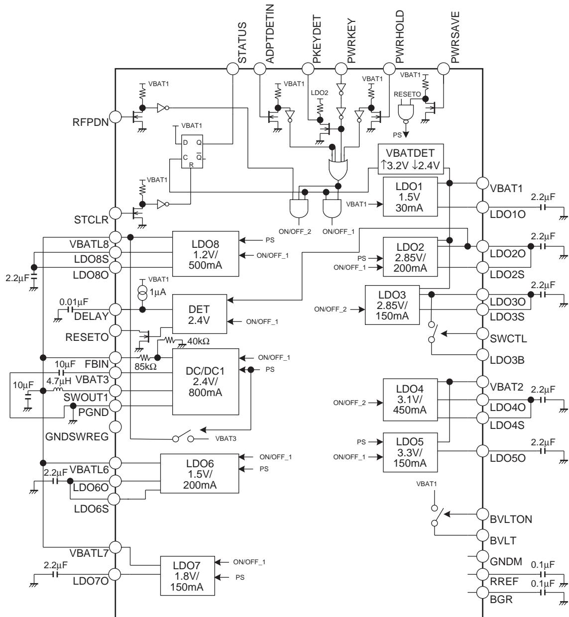
The three power supply pins VBAT1, VBAT2, and VBAT3 must be shorted together externally.
