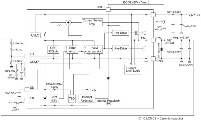
•C1,C8,C5,C9 = Ceramic capacitor •L1 = CDRH105RNP-100NC (sumida)
