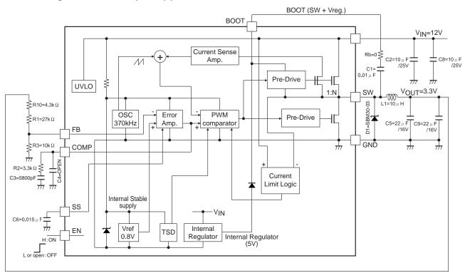
C1,C8,C5,C9 = Ceramic capacitor L1=CDRH105RNP-100NC(sumida)
