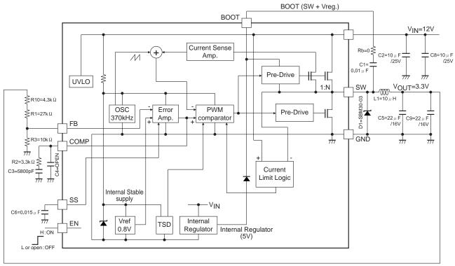
C1,C8,C5,C9 = Ceramic capacitor L1=CDRH105RNP-100NC(sumida)
