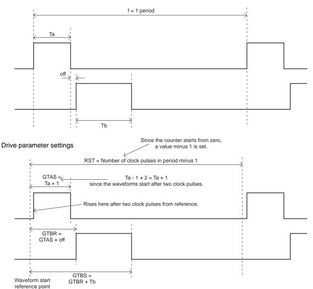
The drive waveforms are set using four parameters: RST, GTAS, GTBR and GTBS.
