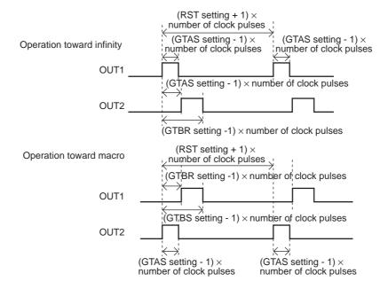
Sequence of initial setting operation ("on" or "off" can be set by the I<sup>2</sup>C settings.) When M/I register =  $00 \rightarrow$  Movement toward infinity position
