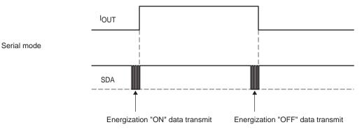
In the serial mode, energization is started by setting energization ON with serial data and stopped by setting it OFF.
