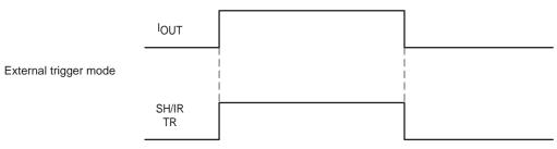
In the external trigger mode, energization is started on a rising edge of the SH/IR TR signal and stopped on the falling edge.
