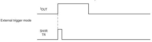
Energization starts on a rising edge of the SH/IR TR signal in the external trigger mode.
