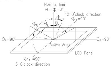
2. Test equipment setup: After stabilizing and leaving the panel alone at a driven temperature for 10 minutes, the measurement should be executed. Measurement should be executed in a stable, windless, and dark room. Optical specifications are measured by Topcon BM-7(BM-5) luminance meter 1.0° field of view at a distance of 50cm and normal direction.
