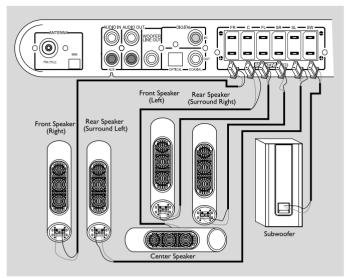
Connect the supplied speaker system using the supplied speaker cables by matching the colours of the jacks and speaker plugs. Fully insert the plugs of speaker wire into the jacks on the DVD system.
