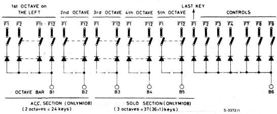
Note: The switch "OPEN" corresponds to "KEY NOT PRESSED" or "CONTROL IN THE FIRST CONDITION" (see the drawing "MATRIX ORGANIZATION").
