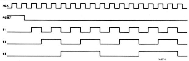
Note: MCK is the master clock input (matrix scanning),  $\varphi 1$ ,  $\varphi 2$ ,  $\varphi 3$  are internal phases to generate  $\overline{F1} \div \overline{F12}$ .
