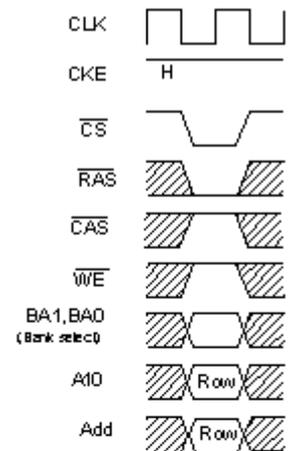
Fig. 2 Row address strobe and bank active command
