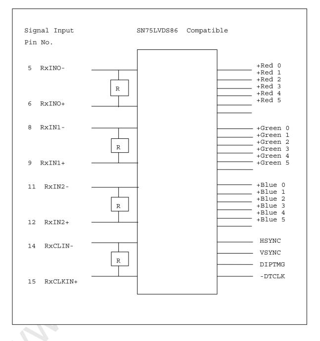
The module uses a 100 ohms resistor between positive and negative data lines of each receiver input.
