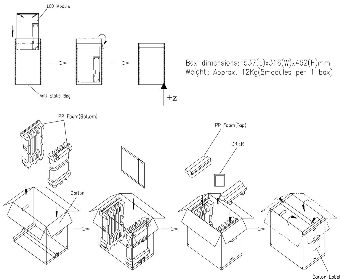
**Figure. 8-1 Packing method**
