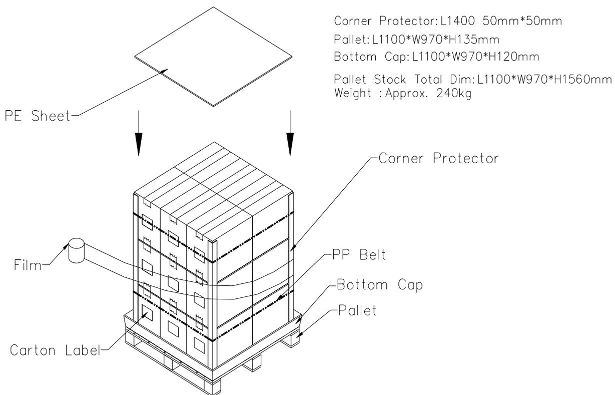
**Figure. 8-2 Packing method**
