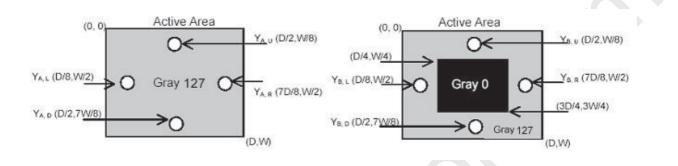
Note 9: Test Patern: Subchecker Pattern measured by TOPCON SR-3
