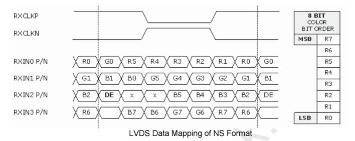
Note1: Normally, DE, VS, HS on EVEN channel are not used. Note2: 8-bits signal input.
