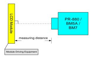
\*\*' EZ Contrast is different measurement tool with very close viewing distance.
