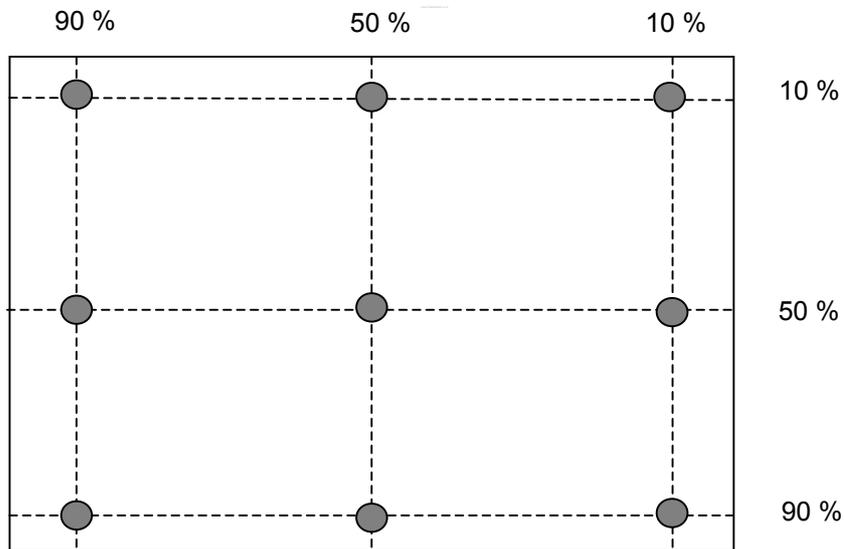
$$\text{Uniformity} = \frac{\text{Minimum Luminance in 9 points (1-9)}}{\text{Maximum Luminance in 9 Points (1-9)}} \times 100\%$$
