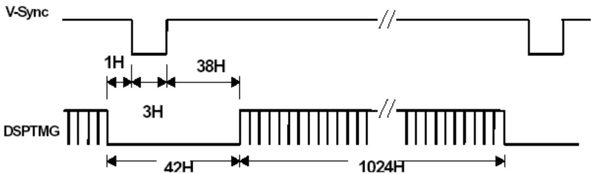
Basically, interface timings described here is not actual input timing of LCD module but output timing of SN75LVDS82DGG (Texas Instruments) or equivalent.
