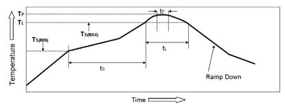
The Pb Free Process-Package Peak Reflow Temperature is 260°C. Exceeding the maximum soldering temperature could permanently damage the module.
