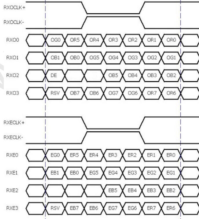
**Note 1:** R/G/B data 7:MSB, R/G/B data 0:LSB      O = "Odd Pixel Data"      E = "Even Pixel Data"
