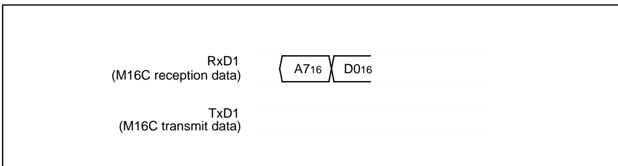
Figure 1.25.27. Timing for erasing all unlocked blocks
