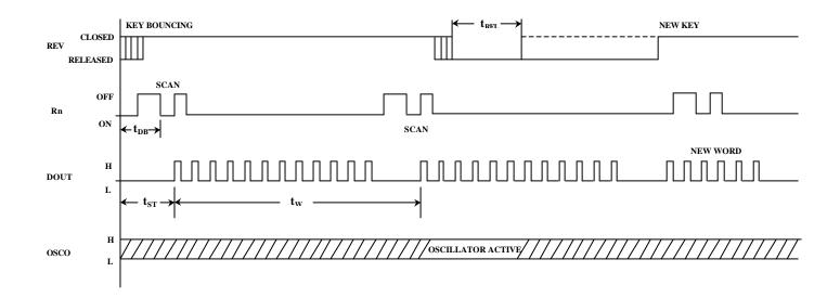
Figure 3 : Multiple key-stroke sequence. Scanrate multiple key-stroke :  $t_{SM} = 8$  TO 10 X TO
