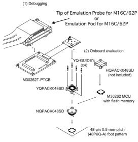
•: No. 1 pin position Be sure to align the pins.
