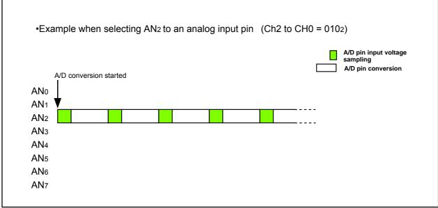
Figure 15.8 Operation Example in Repeat Mode
