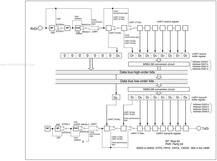
Figure 14.2 Block diagram of UARTi (i = 0, 1) transmit/receive unit
