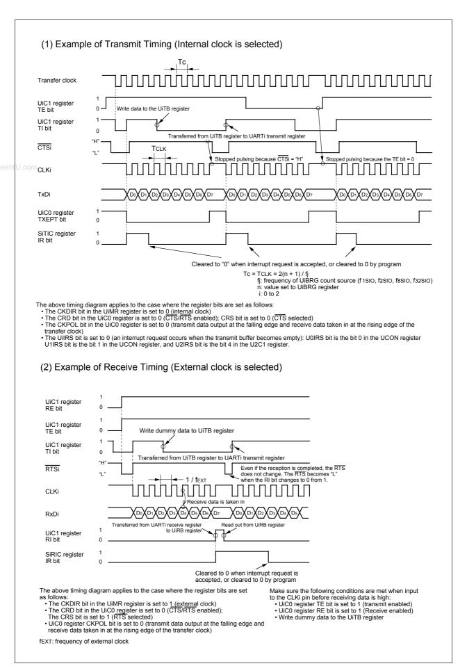
Figure 14.10 Typical transmit/receive timings in clock synchronous serial I/O mode
