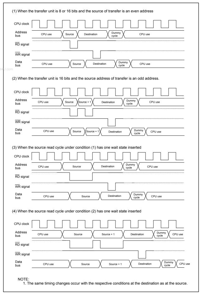
Figure 11.5 Transfer Cycles for Source Read
