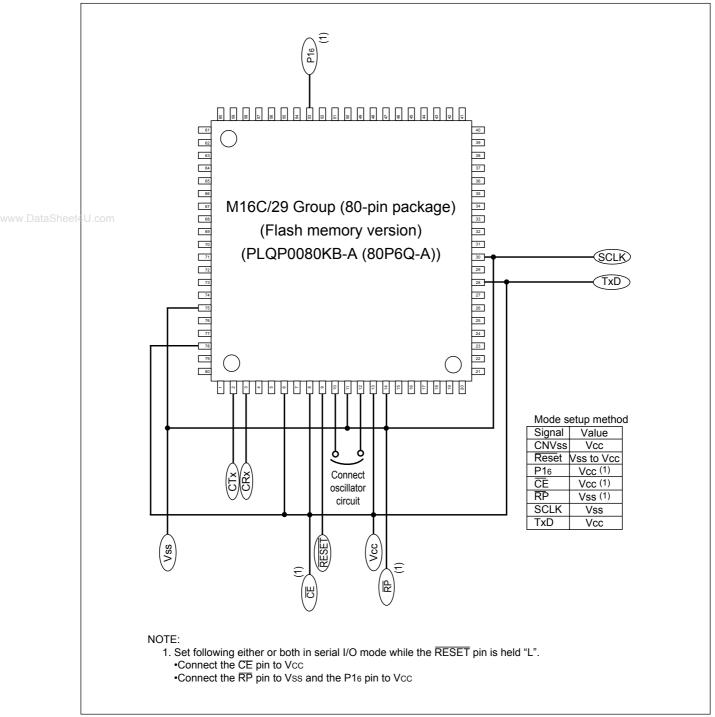
Figure 20.20 Pin Connections for CAN I/O Mode (2)
