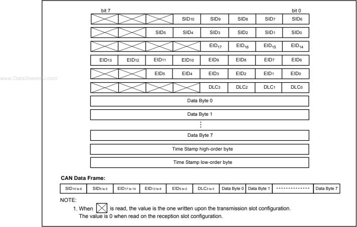
Figure 17.2 Bit Mapping in Byte Access
