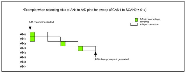
Figure 15.16 Operation Example in Simultaneous Sample Sweep Mode
