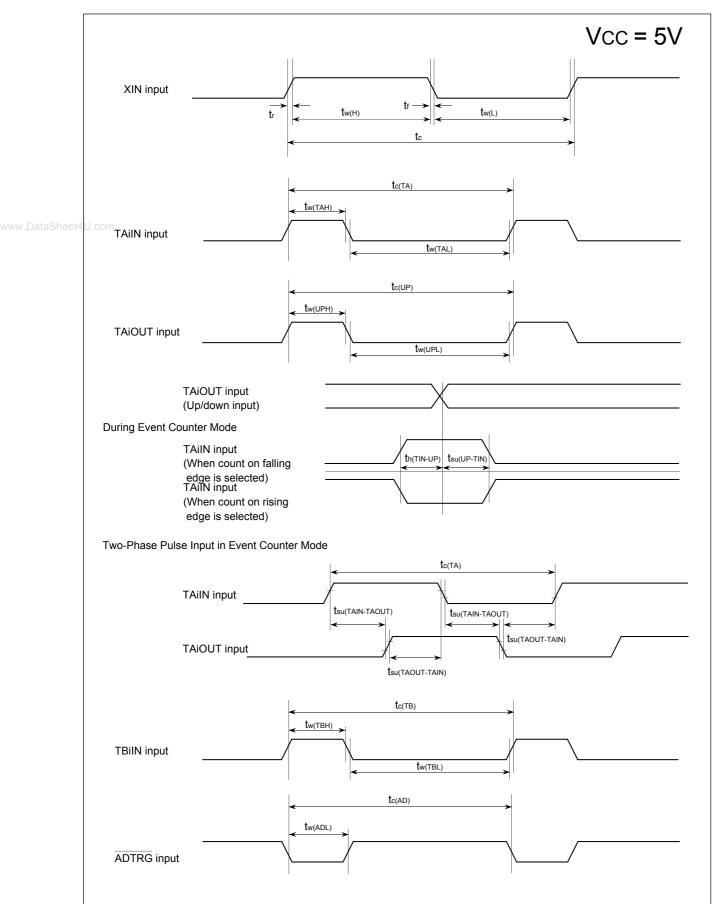
Figure 21.1 Timing Diagram (1)
