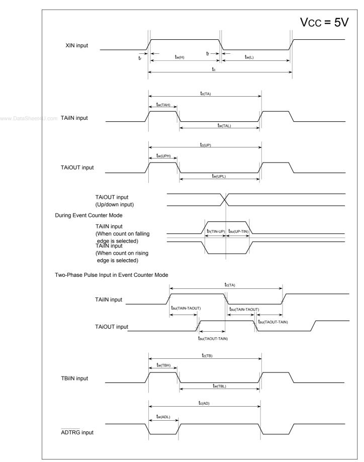
Figure 21.7 Timing Diagram (1)
