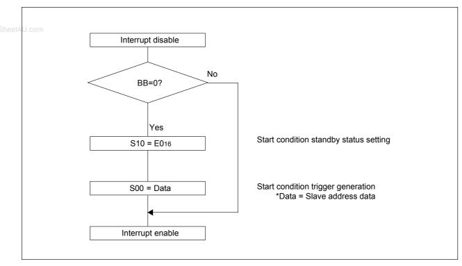
Figure 16.14 Start condition generation flow chart
