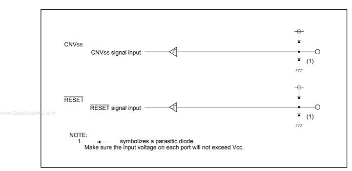
Figure 19.5 I/O Pins
