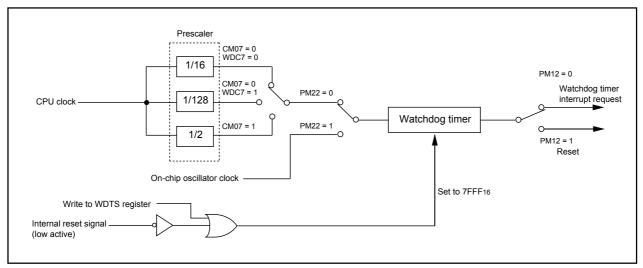
Figure 10.1 Watchdog Timer Block Diagram
