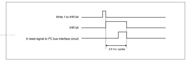
Figure 16.10 The timing of reset to the I<sup>2</sup>C bus interface circuit
