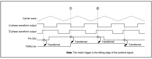
Figure 12.35 Usage Example of Position-data-retain Function (U phase)
