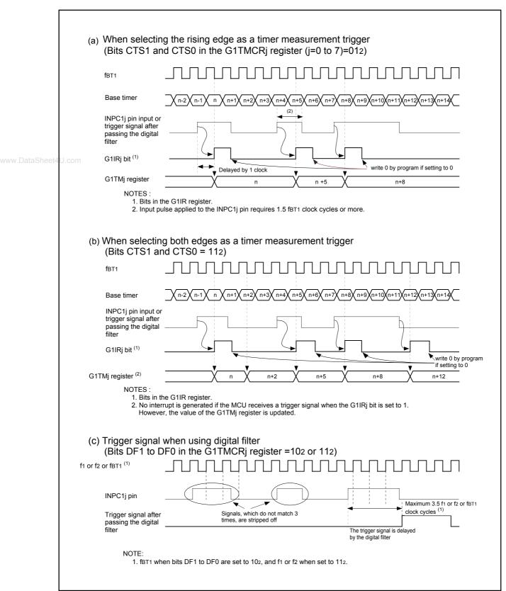
Figure 13.20 Time Measurement Function (2)
