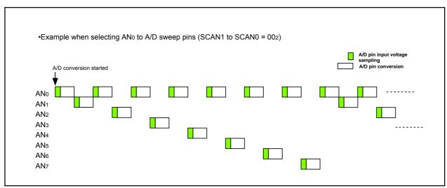
Figure 15.14 Operation Example in Repeat Sweep Mode 1
