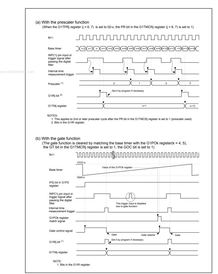
Figure 13.21 Prescaler Function and Gate Function
