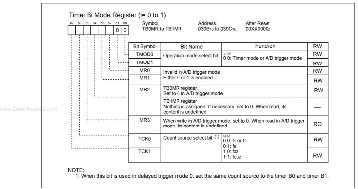
Figure 12.23 TBiMR Register in A/D Trigger Mode
