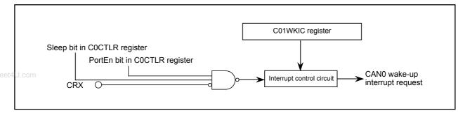
Figure 9.13 CAN0 Wake-up Interrupt Block Diagram
