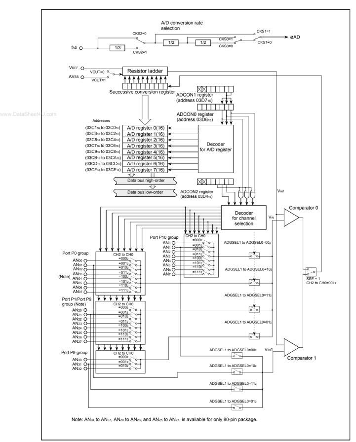
Figure 15.1 A/D Converter Block Diagram
