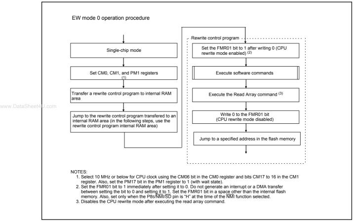
Figure 20.8 Setting and Resetting of EW Mode 0
