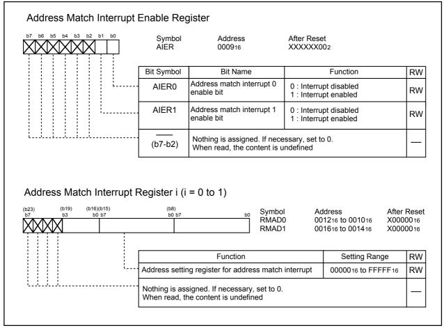
Figure 9.14 AIER Register, RMAD0 and RMAD1 Registers
