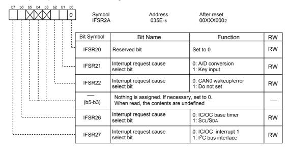
Figure 9.4 IFSR Register and IFSR2A Register
