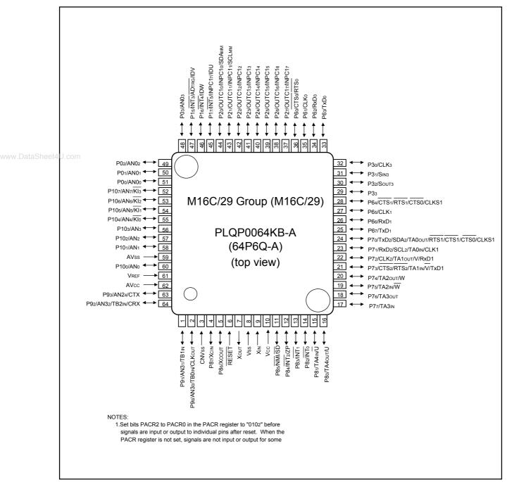
Figure 1.9 Pin Assignment (Top View) of 64-Pin Package
