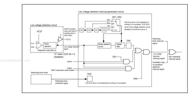
Figure 5.8 Low Voltage Detection Interrupt Generation Block
