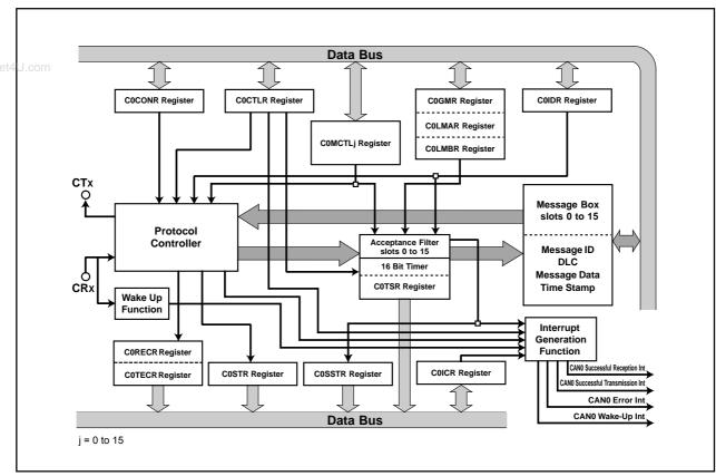
Figure 17.1 Block Diagram of CAN Module
