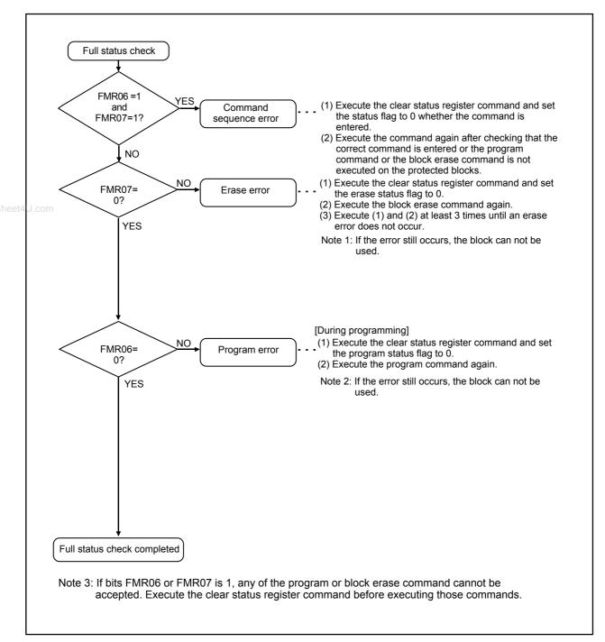
Figure 20.14 Full Status Check and Handling Procedure for Each Error
