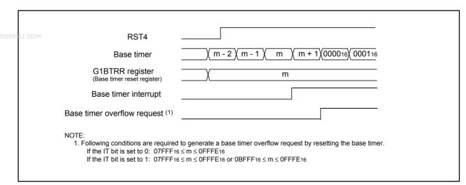
Figure 13.15 Base Timer Reset operation by Base Timer Reset Register
