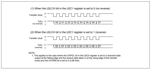
Figure 14.13 Serial data logic switch timing
