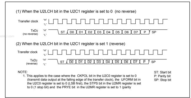
Figure 14.19 Serial Data Logic Switching
