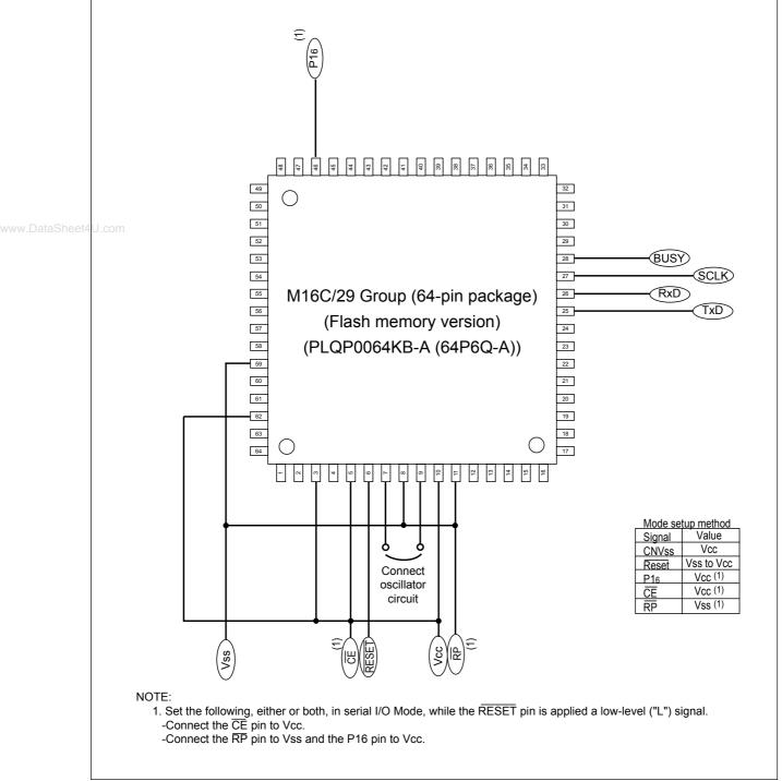
Figure 20.15 Pin Connections for Serial I/O Mode (1)
