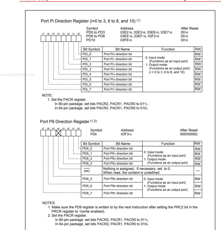
Figure 19.6 PD0 to PD3 and PD6 to PD10 Registers
