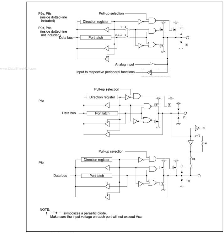
Figure 19.4 I/O Ports (4)
