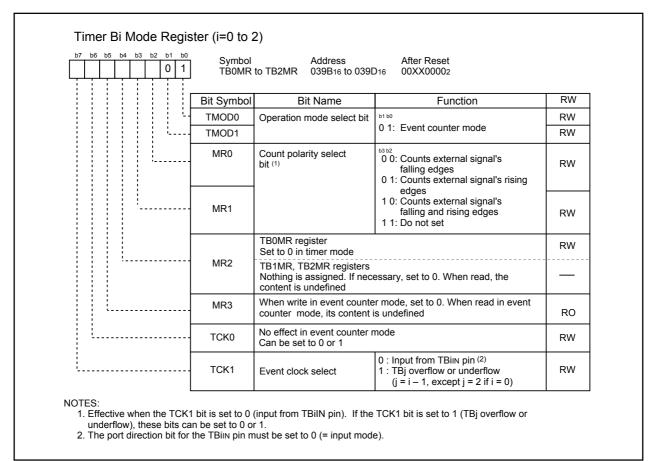
Figure 12.19 TBiMR Register in Event Counter Mode
