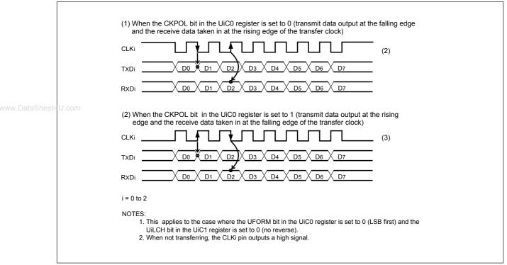
Figure 14.11 Polarity of transfer clock
