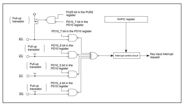
Figure 9.12 Key Input Interrupt
