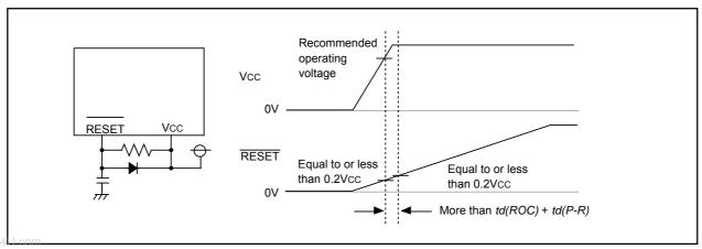
Figure 5.1 Example Reset Circuit
