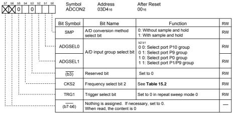
Figure 15.13 ADCON0 to ADCON2 Registers in Repeat Sweep Mode 0
