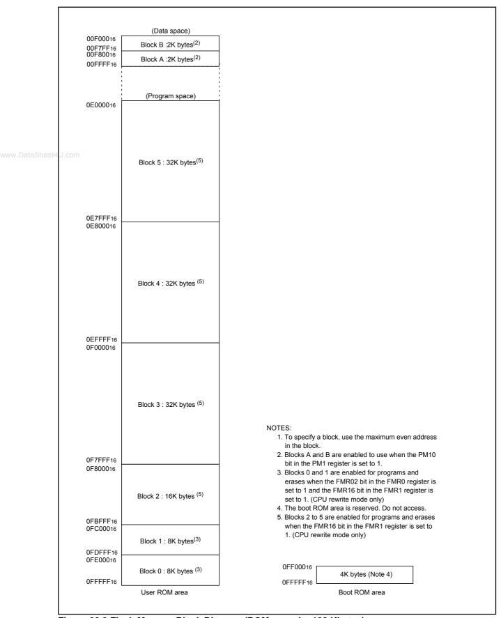
Figure 20.3 Flash Memory Block Diagram (ROM capacity 128 Kbytes)
