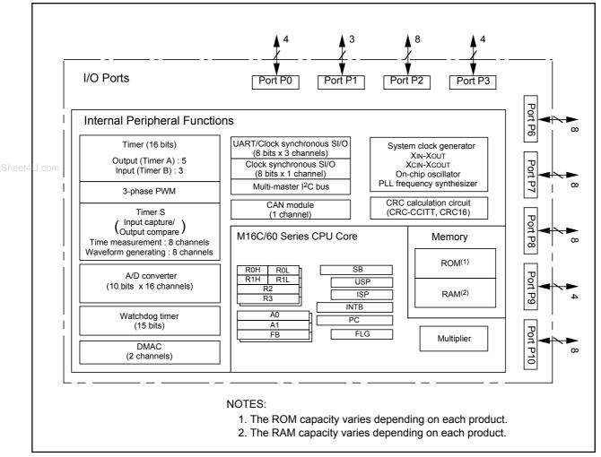
Figure 1.2 M16C/29 Group, 64-Pin Block Diagram
