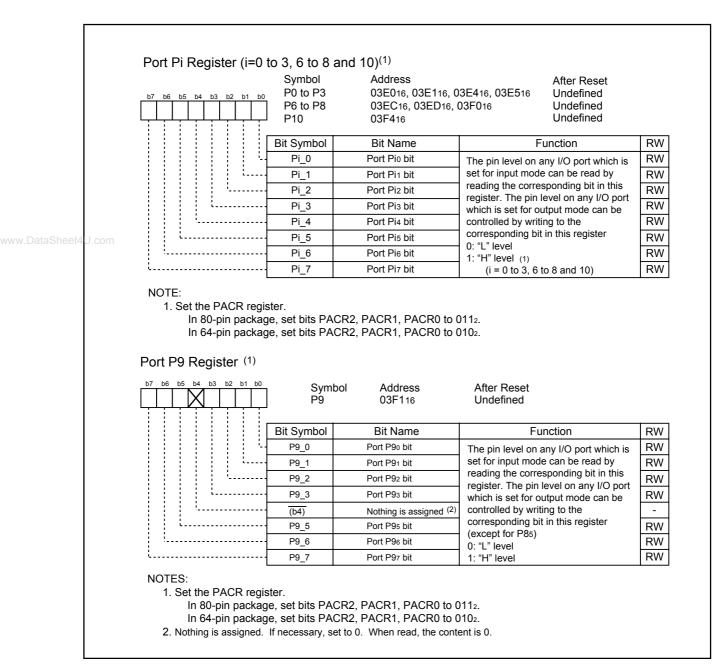
Figure 19.7 P0 to P3 and P6 to P10 Registers
