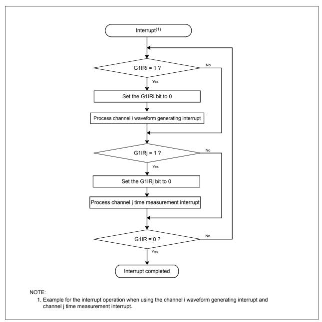
Figure 22.3 IC/OC Interrupt i Flow Chart
