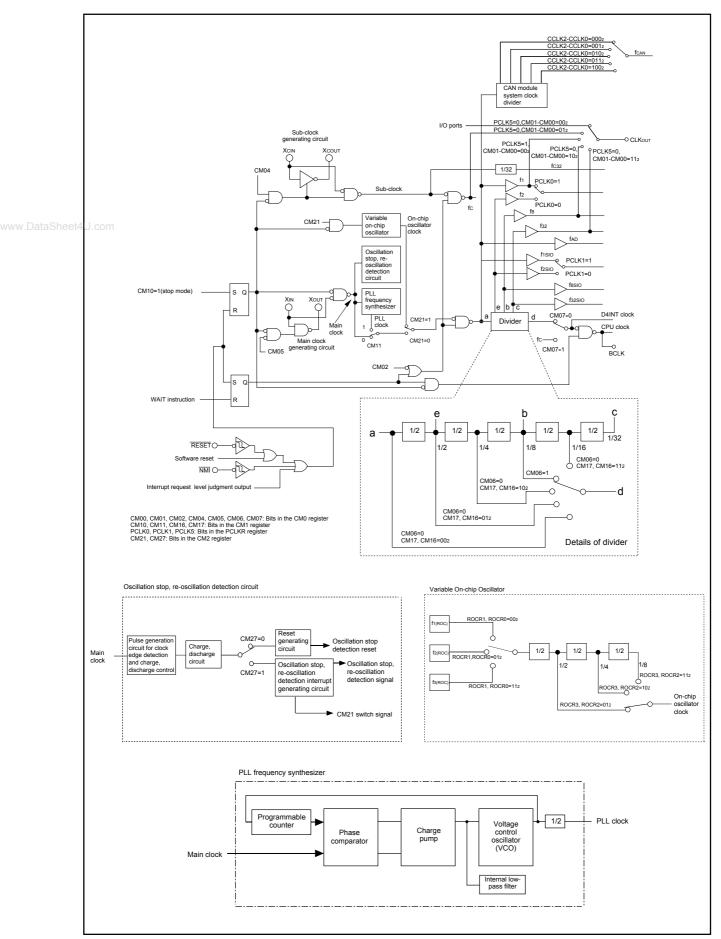
Figure 7.1 Clock Generation Circuit
