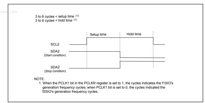
Figure 14.24 Detection of Start and Stop Condition
