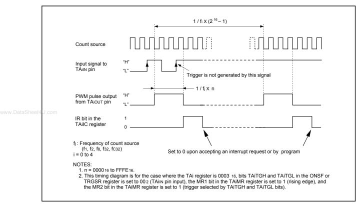
Figure 12.13 Example of 16-bit Pulse Width Modulator Operation
