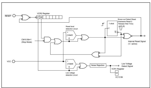
Figure 5.4 Voltage Detection Circuit Block
