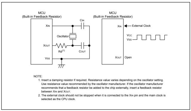
Figure 7.8 Examples of Main Clock Connection Circuit
