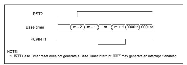
Figure 13.17 Base Timer Reset operation by INT1
