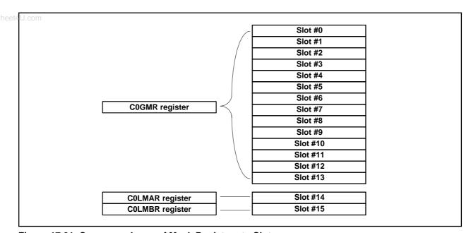
Figure 17.21 Correspondence of Mask Registers to Slots
