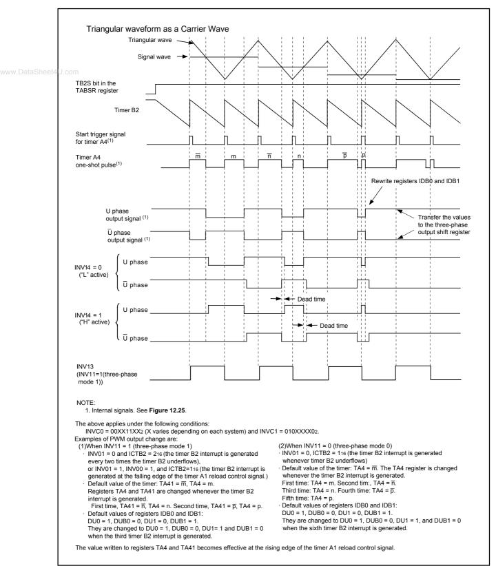
Figure 12.33 Triangular Wave Modulation Operation
