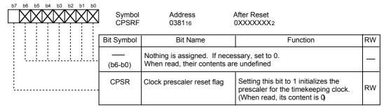
Figure 12.6 ONSF Register, TRGSR Register, and CPSRF Register
