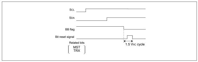
Figure 16.21 The bit reset timing (The STOP condition detection)
