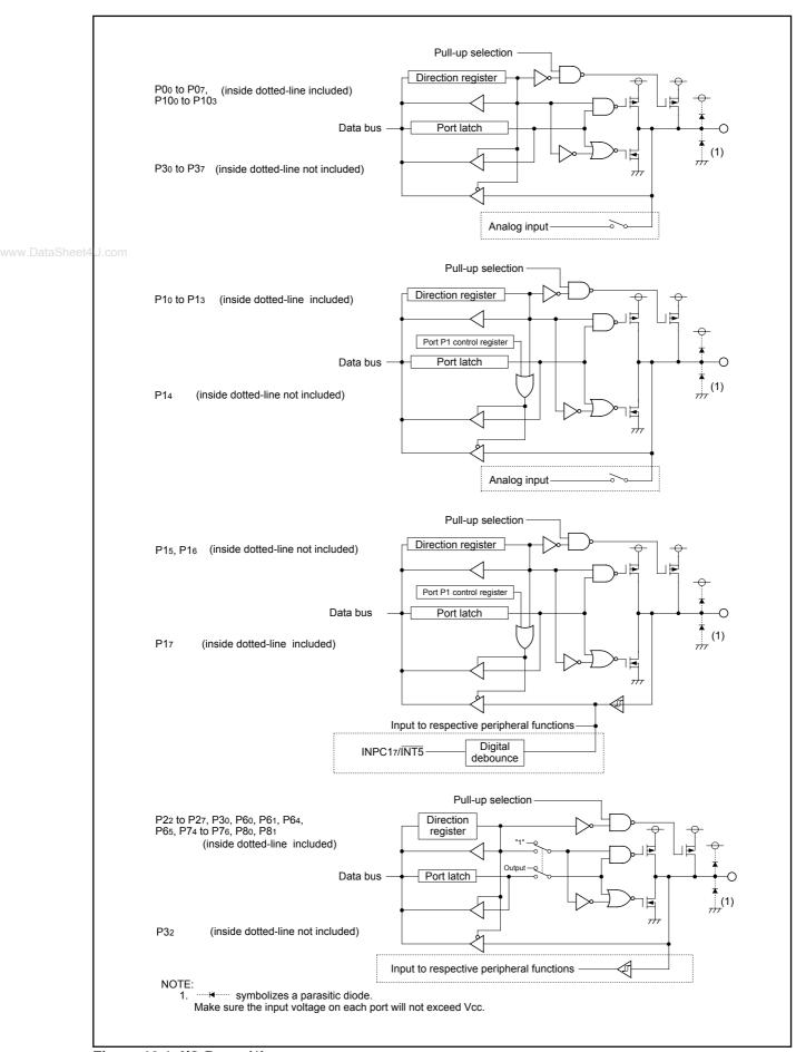
Figure 19.1 I/O Ports (1)
