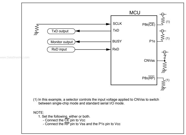
Figure 20.18 Circuit Application in Standard Serial I/O Mode 2
