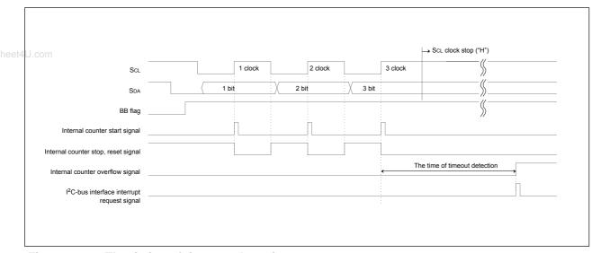
Figure 16.13 The timing of time-out detection
