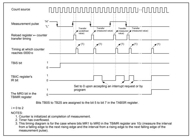
Figure 12.22 Operation timing when measuring a pulse width
