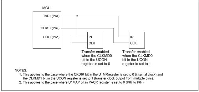
Figure 14.14 Transfer Clock Output From Multiple Pins
