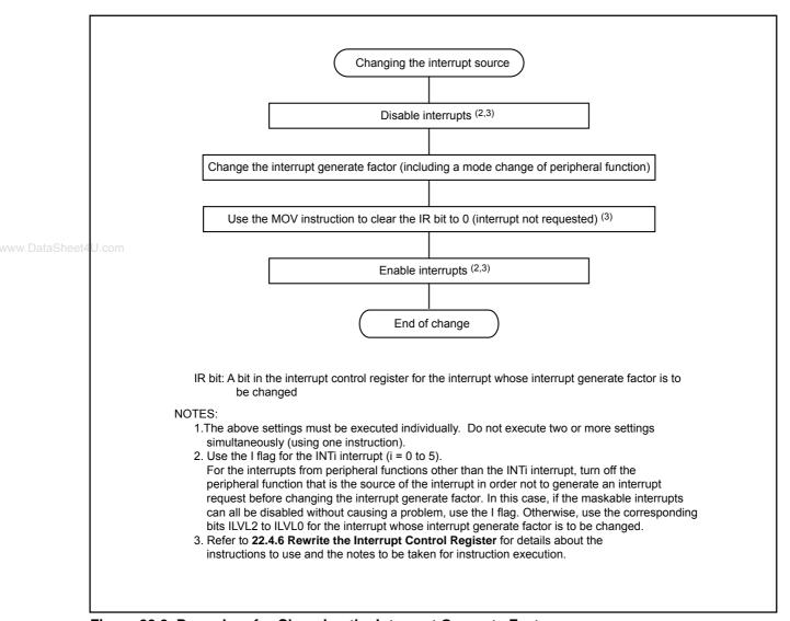
Figure 22.2 Procedure for Changing the Interrupt Generate Factor
