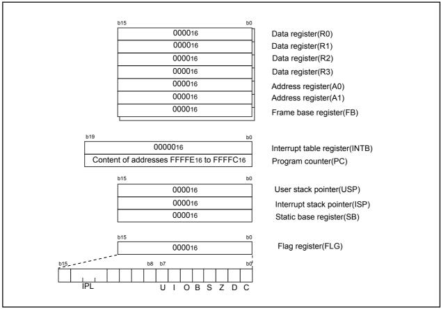
Figure 5.3 CPU Register Status After Reset
