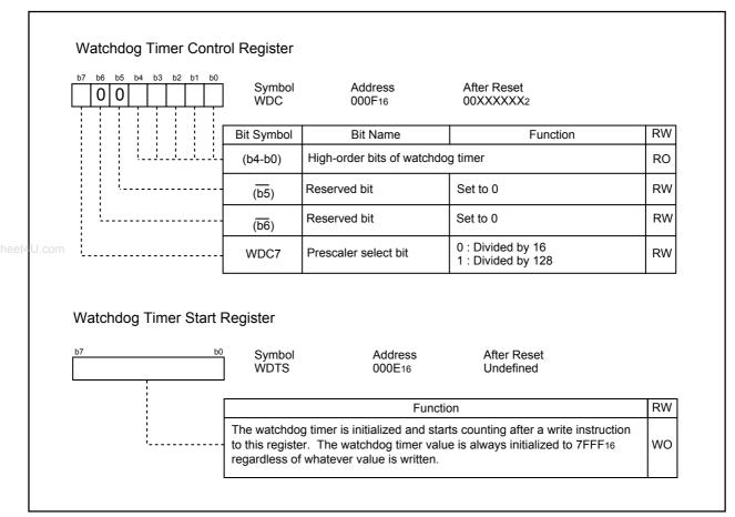
Figure 10.2 WDC Register and WDTS Register
