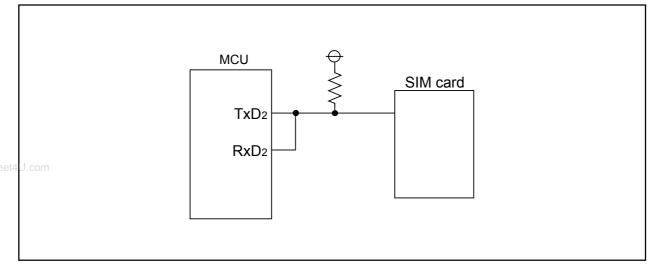
Figure 14.32 SIM Interface Connection
