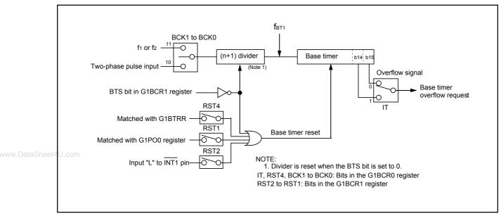
Figure 13.11 Base Timer Block Diagram
