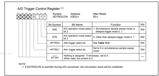
Figure 15.18 ADTRGCON Register in Simultaneous Sample Sweep Mode
