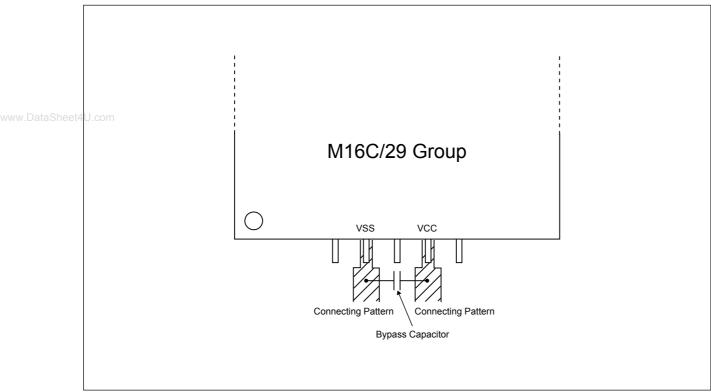
Figure 22.8 Bypass Capacitor Connection
