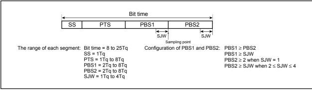
Figure 17.20 Bit Timing
