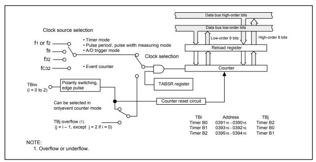
Figure 12.15 Timer B Block Diagram
