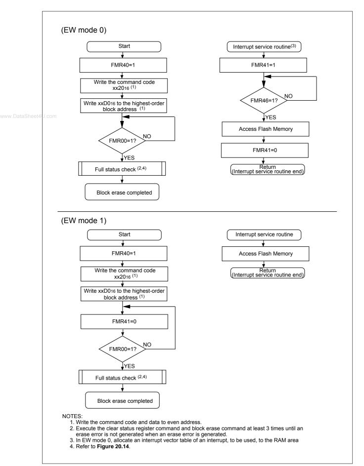
Figure 20.13 Block Erase Command (at use erase suspend)
