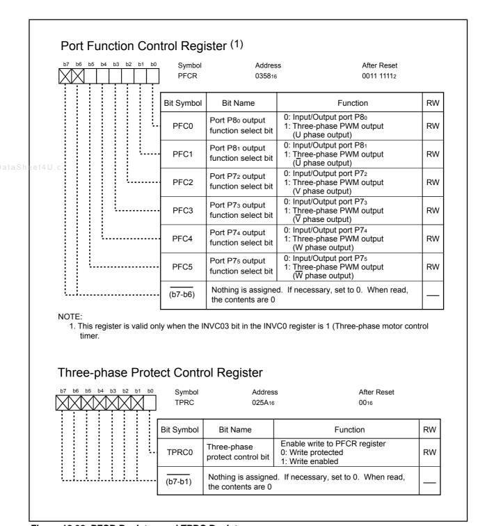
Figure 12.38 PFCR Register, and TPRC Register
