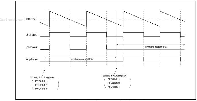
Figure 12.37 Usage Example of Three-phse/Port Output Switch Function
