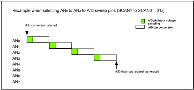
Figure 15.10 Operation Example in Single Sweep Mode
