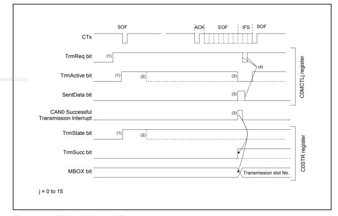
Figure 17.26 Timing of Transmit Sequence
