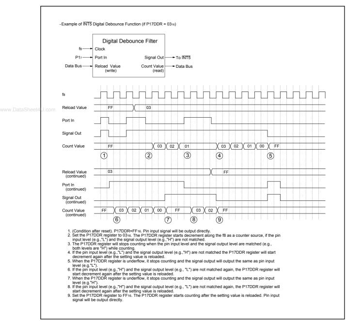
Figure 19.12 Functioning of Digital Debounce Filter
