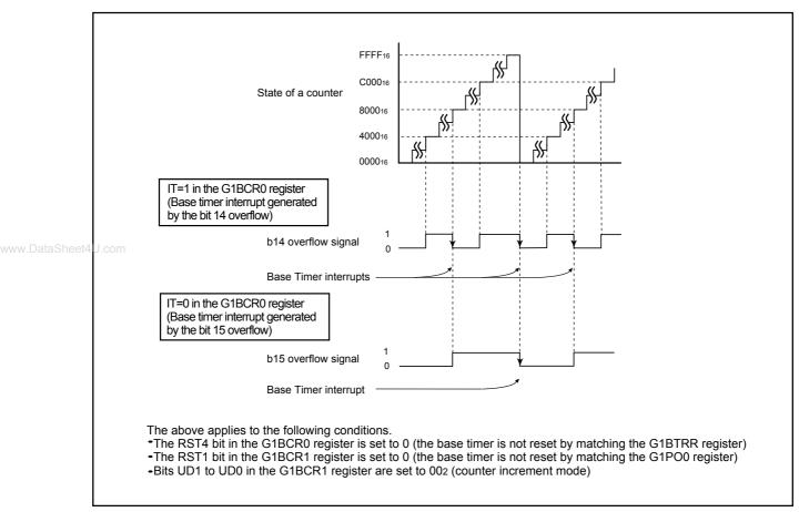
Figure 13.12 Counter Increment Mode
