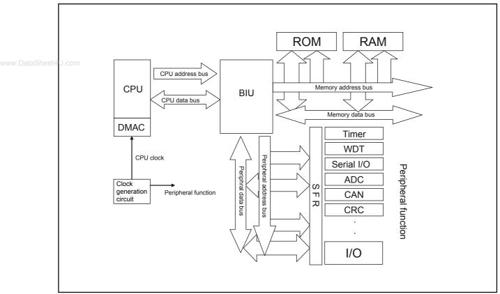
Figure 6.3 Bus Block Diagram
