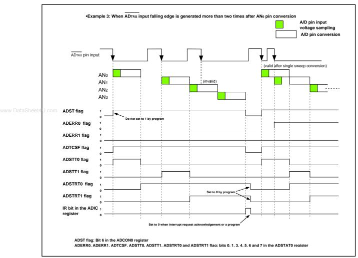
Figure 15.26 Each Flag Operation in ADSTAT0 Register Associated with the Operation Example in Delayed Trigger Mode 1 (2)
