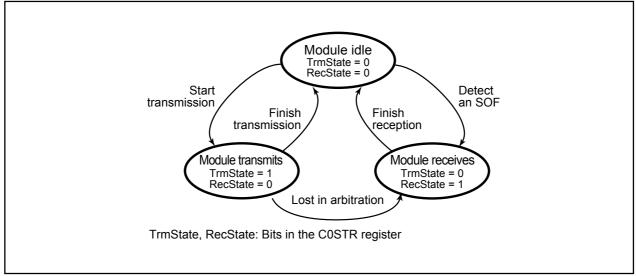
Figure 17.18 Sub Modes of CAN Operating Mode
