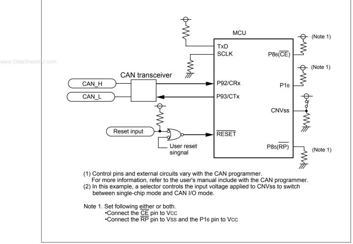
Figure 20.21 Circuit Application in CAN I/O Mode
