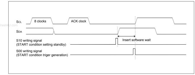
Figure 16.24 The time of generation of RESTART condition
