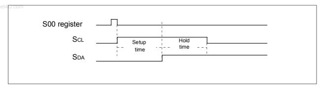
Figure 16.17 Stop condition generation timing diagram
