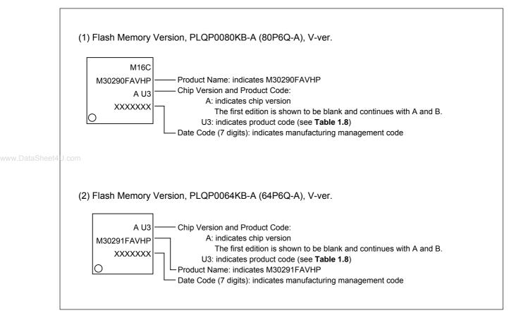
Figure 1.6 Marking Diagrams of Flash Memory Version - M16C/29 Group V-ver. (Top View)
