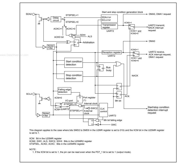
Figure 14.22 I<sup>2</sup>C bus mode Block Diagram
