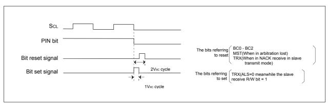
Figure 16.23 Bit set/reset timing (at the completion of data transfer)
