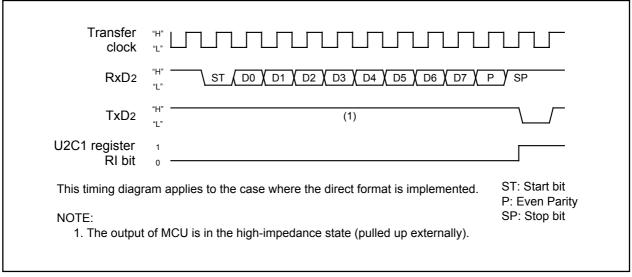
Figure 14.33 Parity Error Signal Output Timing
