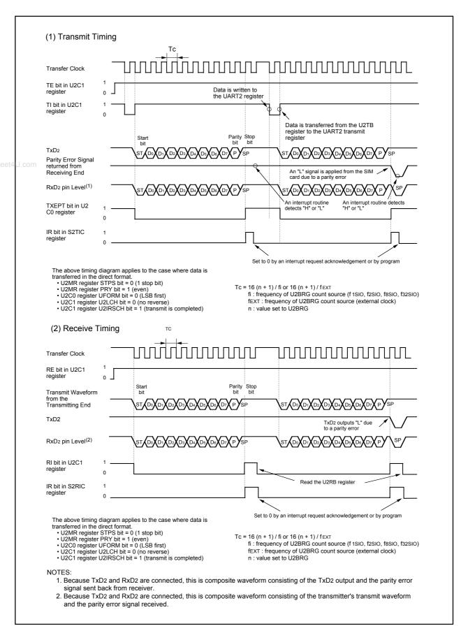
Figure 14.31 Transmit and Receive Timing in SIM Mode
