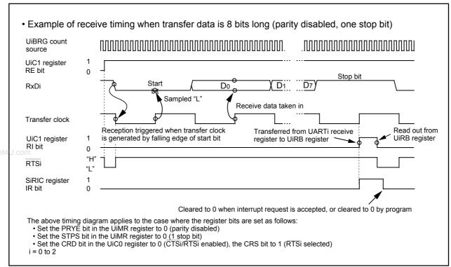
Figure 14.17 Receive Operation
