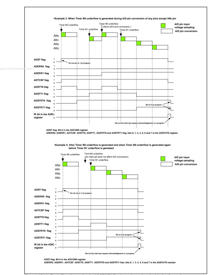
Figure 15.21 Each Flag Operation in ADSTAT0 Register Associated with the Operation **Example in Delayed Trigger Mode 0 (2)**
