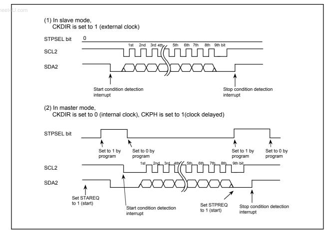
Figure 14.25 STSPSEL Bit Functions
