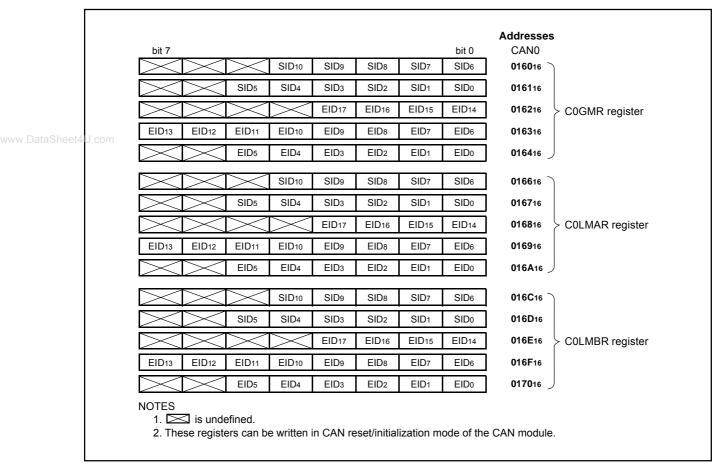
Figure 17.4 Bit Mapping of Mask Registers in Byte Access
