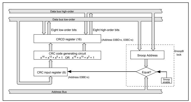
Figure 18.1 CRC circuit block diagram
