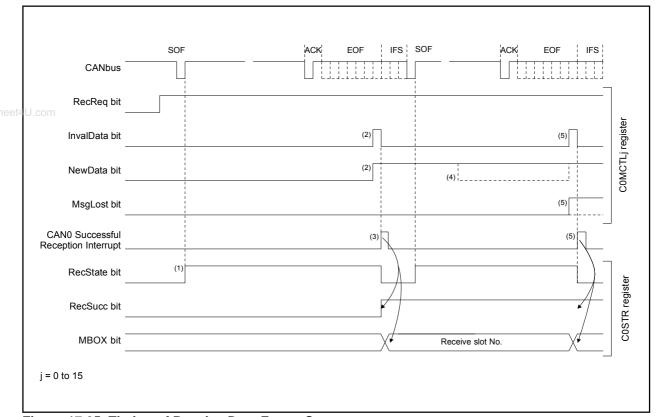
Figure 17.25 Timing of Receive Data Frame Sequence
