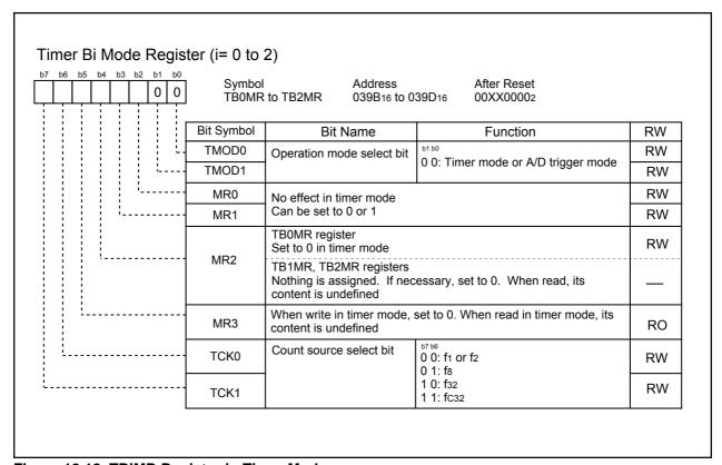
Figure 12.18 TBiMR Register in Timer Mode
