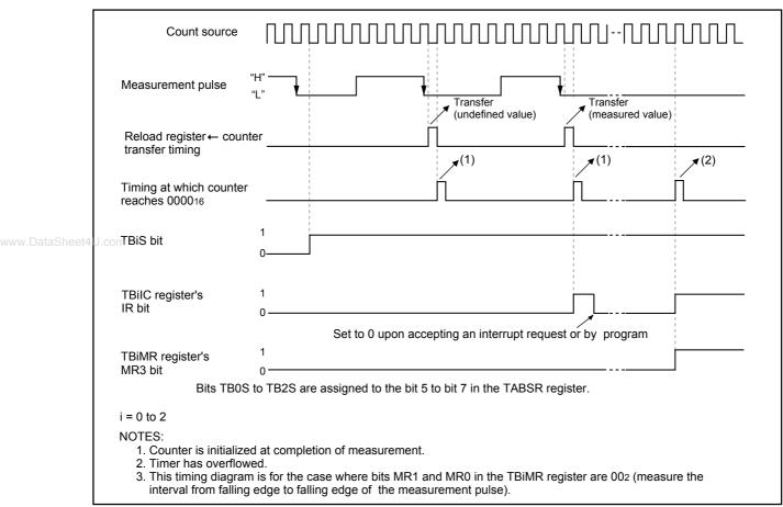
Figure 12.21 Operation timing when measuring a pulse period
