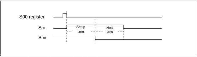
Figure 16.16 Start condition generation timing diagram
