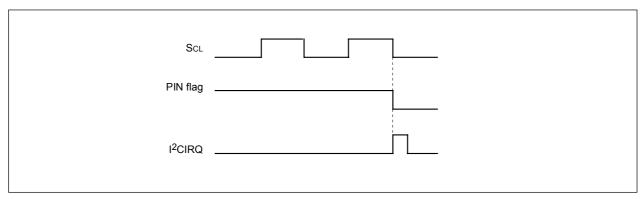
Figure 16.11 Interrupt request signal generation timing
