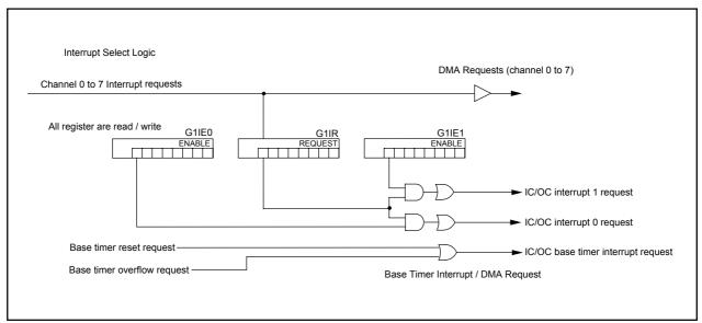
Figure 13.18 IC/OC Interrupt and DMA request generation
