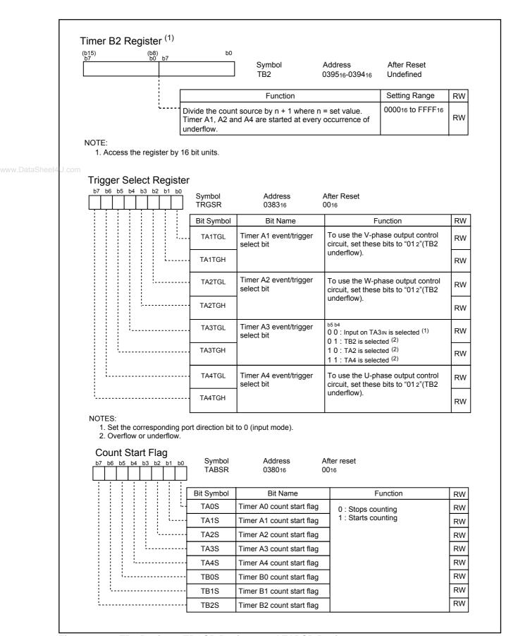
Figure 12.31 TB2 Register, TRGSR Register, and TABSR Register
