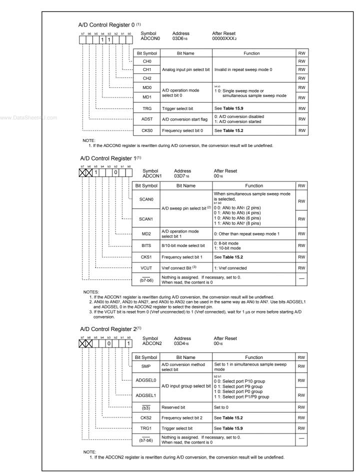
Figure 15.17 ADCON0 to ADCON2 Registers in Simultaneous Sample Sweep Mode
