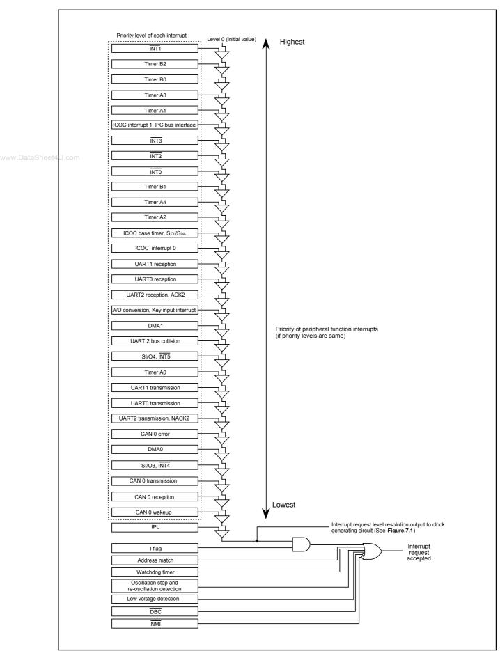
Figure 9.10 Interrupts Priority Select Circuit
