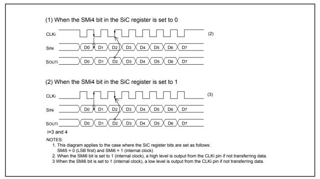
Figure 14.38 Polarity of Transfer Clock
