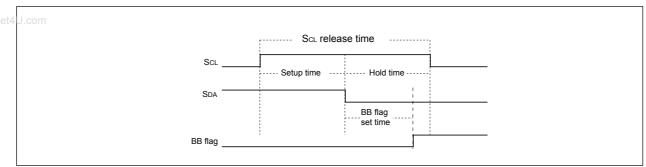
Figure 16.18 Start condition detection timing diagram
