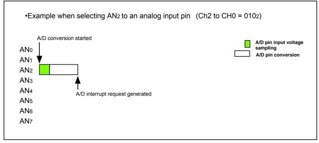
Figure 15.6 Operation Example in One-Shot Mode
