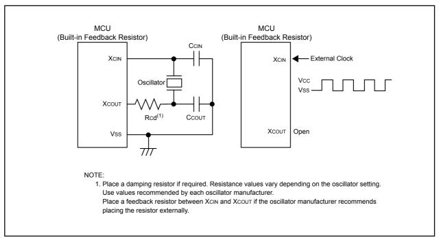
Figure 7.9 Examples of Sub Clock Connection Circuit
