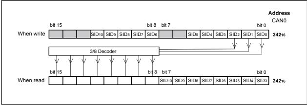
Figure 17.23 Write/read of COAFS Register in Word Access
