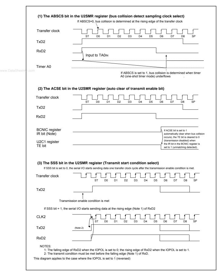
Figure 14.30 Bus Collision Detect Function-Related Bits
