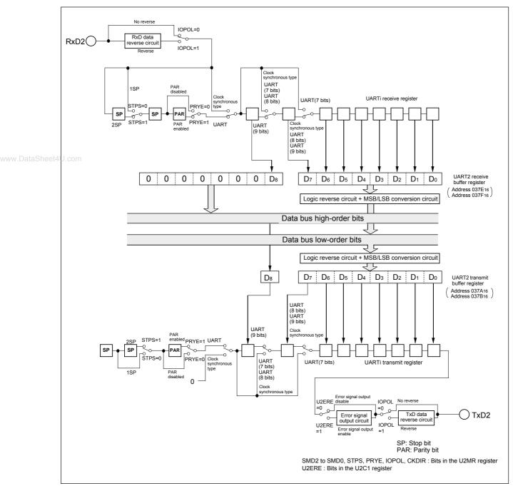
Figure 14.3 Block diagram of UART2 transmit/receive unit
