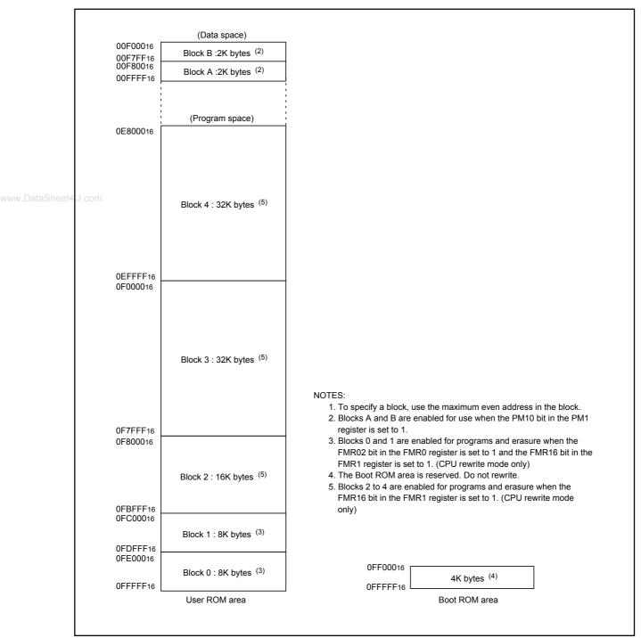
Figure 20.2 Flash Memory Block Diagram (ROM capacity 96 Kbytes)
