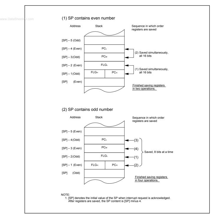
Figure 9.8 Operation of Saving Register
