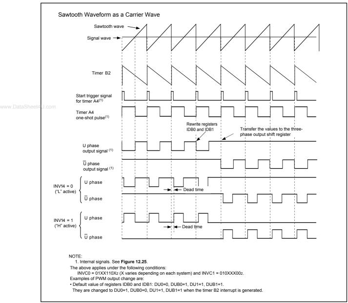
Figure 12.34 Sawtooth Wave Modulation Operation
