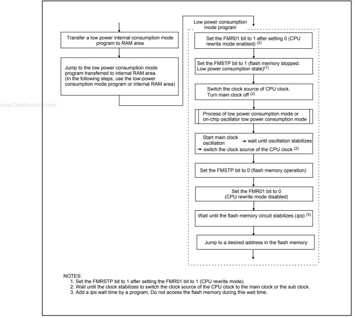
Figure 20.10 Processing Before and After Low Power Dissipation Mode
