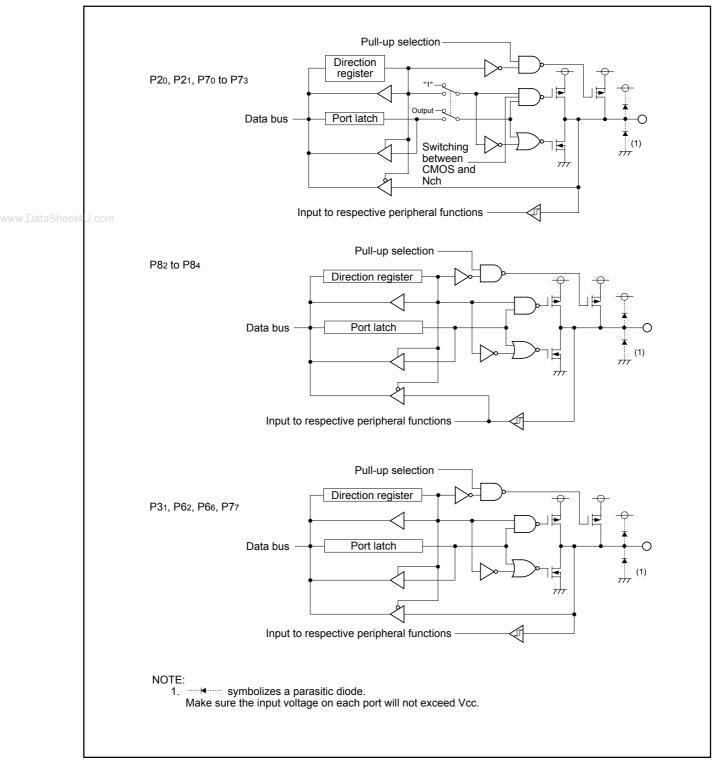
Figure 19.2 I/O Ports (2)
