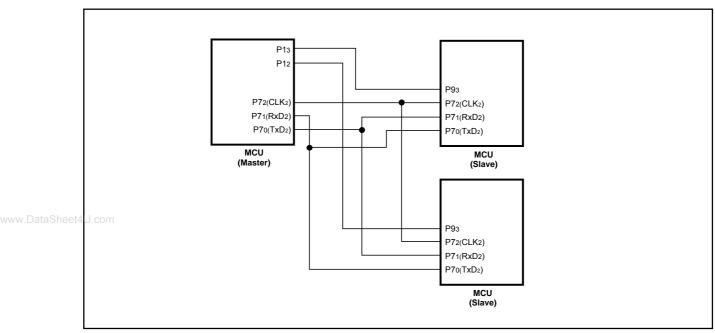
Figure 14.26 Serial Bus Communication Control Example (UART2)
