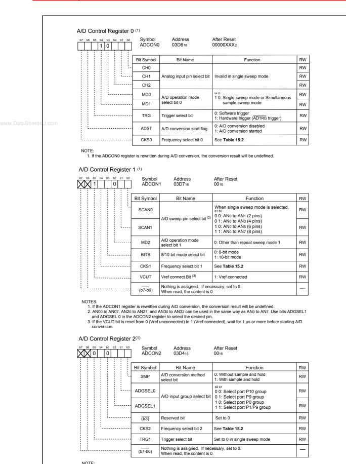
Figure 15.11 ADCON0 to ADCON2 Registers in Single Sweep Mode
