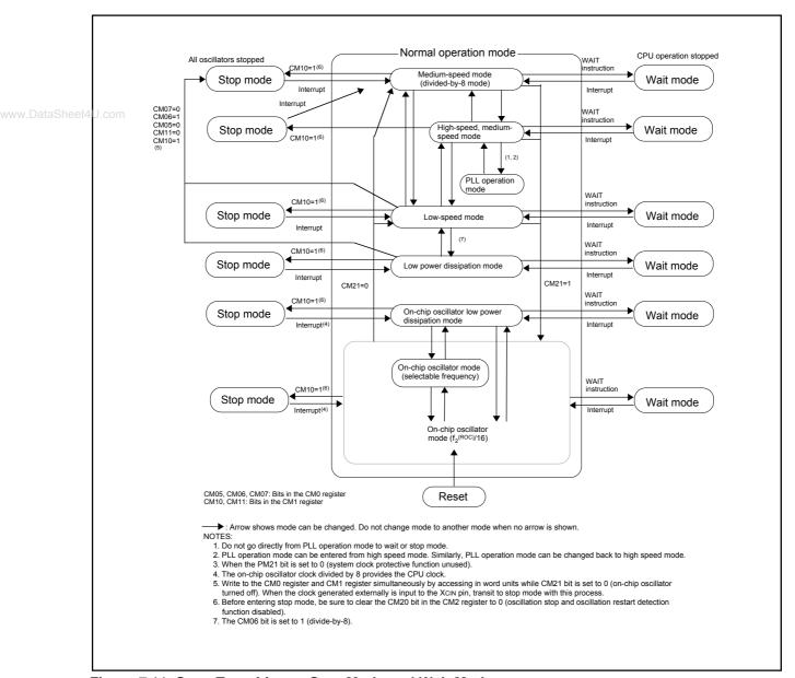
Figure 7.11 State Transition to Stop Mode and Wait Mode
