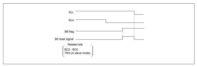
Figure 16.22 The bit reset timing (The START condition detection)
