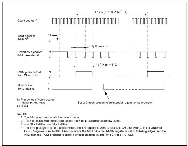
Figure 12.14 Example of 8-bit Pulse Width Modulator Operation
