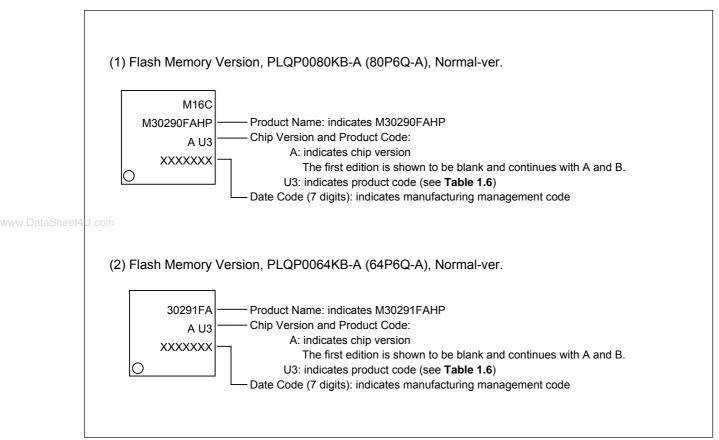
Figure 1.4 Marking Diagrams of Flash Memory Version - M16C/29 Group Normal-ver. (Top View)
