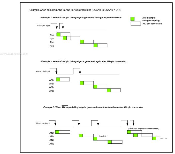
Figure 15.24 Operation Example in Delayed Trigger Mode1
