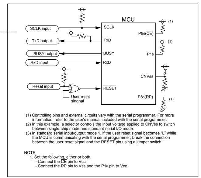
Figure 20.17 Circuit Application in Standard Serial I/O Mode 1
