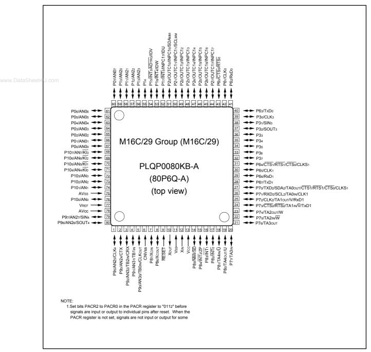
Figure 1.8 Pin Assignment (Top View) of 80-Pin Package
