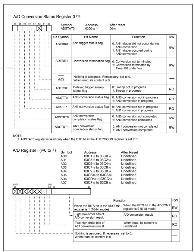
Figure 15.4 ADSTAT0 Register and AD0 to AD7 Registers
