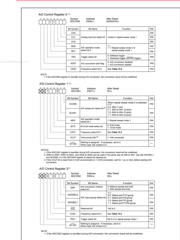
Figure 15.15 ADCON0 to ADCON2 Registers in Repeat Sweep Mode 1
