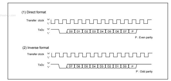
Figure 14.34 SIM Interface Format
