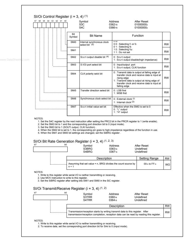
Figure 14.36 S3C and S4C Registers, S3BRG and S4BRG Registers, and S3TRR and S4TRR Registers
