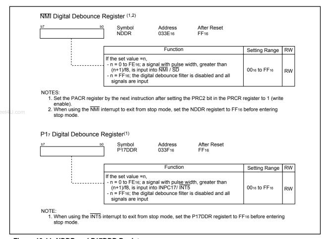
Figure 19.11 NDDR and P17DDR Registers
