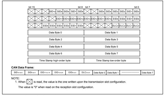
Figure 17.3 Bit Mapping in Word Access
