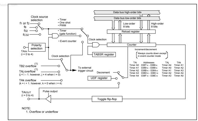
Figure 12.3 Timer A Block Diagram
