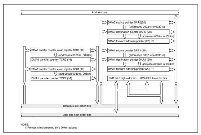
Figure 11.1 DMAC Block Diagram
