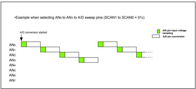
Figure 15.12 Operation Example in Repeat Sweep Mode 0
