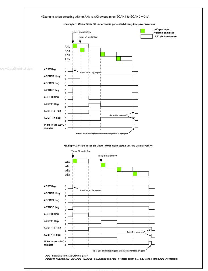
Figure 15.20 Each Flag Operation in ADSTAT0 Register Associated with the Operation Example in Delayed Trigger Mode 0 (1)
