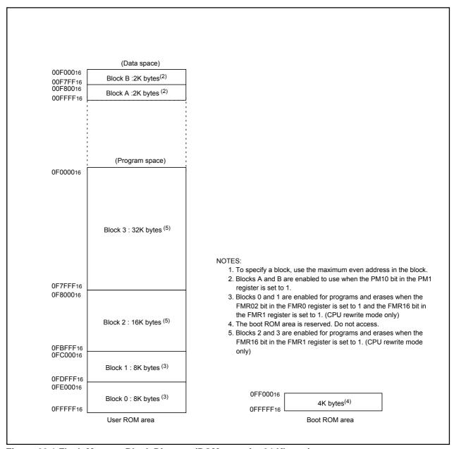
Figure 20.1 Flash Memory Block Diagram (ROM capacity 64 Kbytes)
