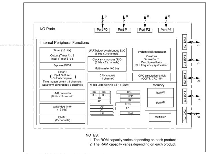
Figure 1.1 M16C/29 Group, 80-Pin Block Diagram
