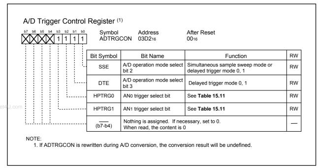
Figure 15.23 ADTRGCON Register in Delayed Trigger Mode 0
