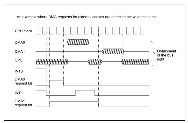
Figure 11.6 DMA Transfer by External Factors
