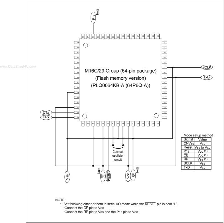
Figure 20.19 Pin Connections for CAN I/O Mode (1)
