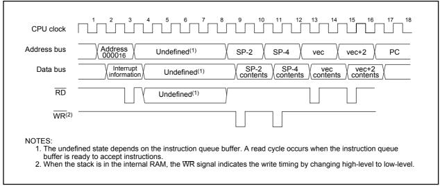
Figure 9.5 Time Required for Executing Interrupt Sequence
