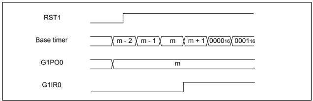
Figure 13.16 Base Timer Reset operation by G1PO0 register
