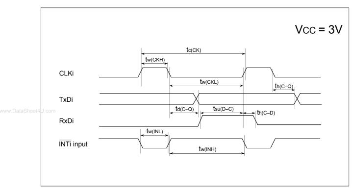
Figure 21.5 Timing Diagram (2)
