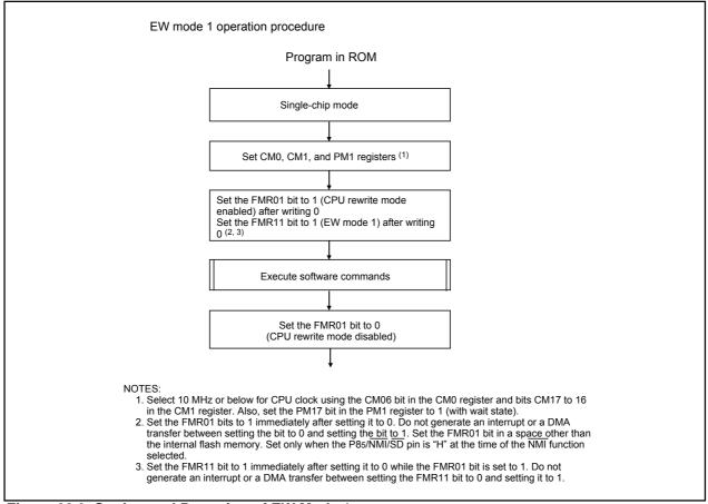
Figure 20.9 Setting and Resetting of EW Mode 1
