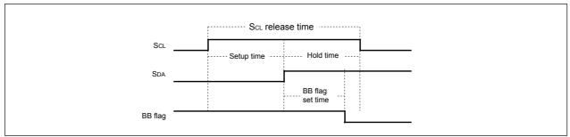
Figure 16.19 Stop condition detection timing diagram
