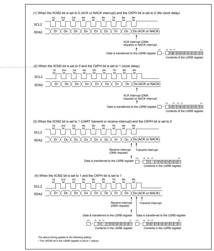
Figure 14.23 Transfer to U2RB Register and Interrupt Timing
