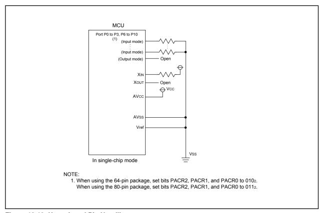
Figure 19.13 Unassigned Pin Handling
