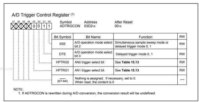
Figure 15.28 ADTRGCON Register in Delayed Trigger Mode 1
