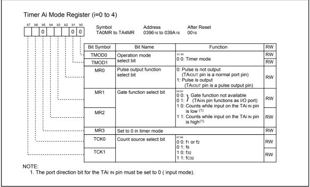
Figure 12.7 Timer Ai Mode Register in Timer Mode
