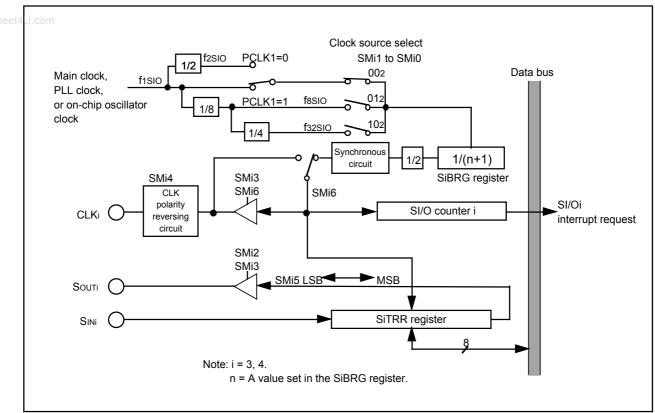
Figure 14.35 SI/O3 and SI/O4 Block Diagram
