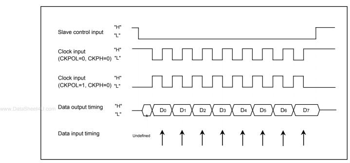
Figure 14.28 Transmission and Reception Timing (CKPH=0) in Slave Mode (External Clock)
