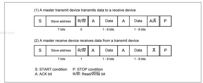
Figure 16.20 Address data communication format
