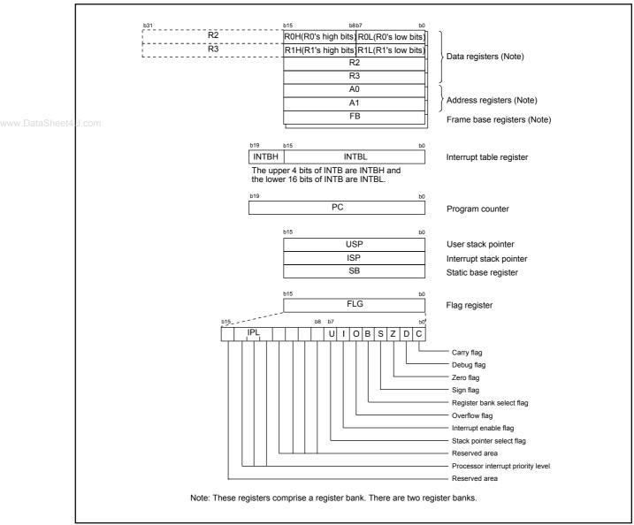
Figure 2.1. Central Processing Unit Register
