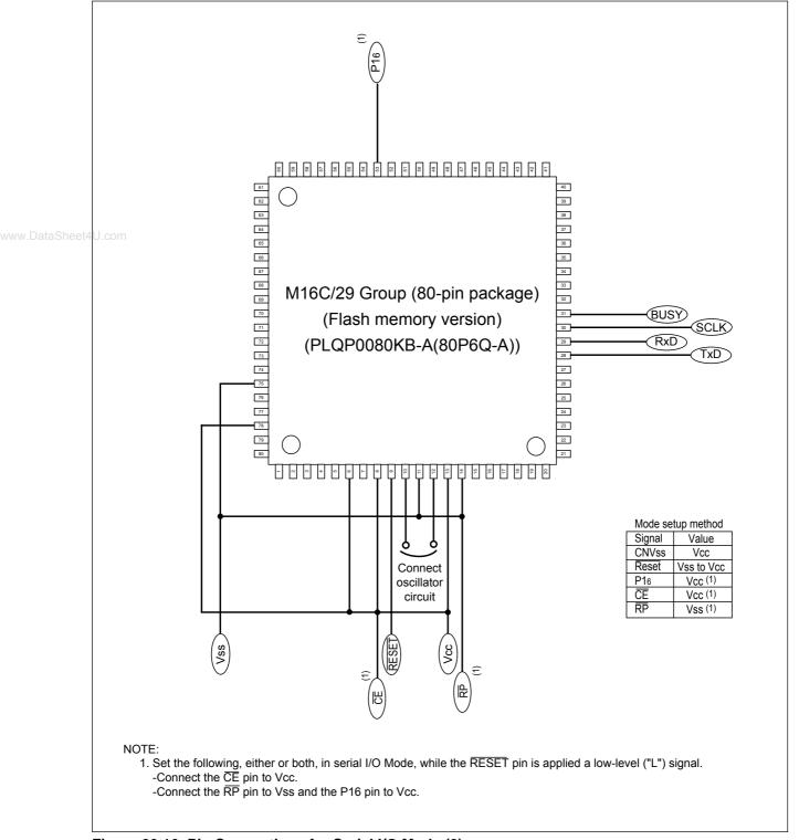
Figure 20.16 Pin Connections for Serial I/O Mode (2)
