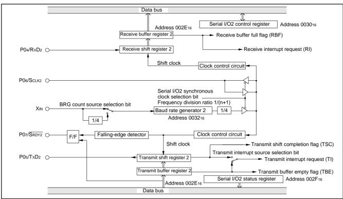
Fig. 63 Block diagram of clock synchronous serial I/O2
