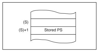
Fig. 2 Stack memory contents after PHP instruction execution
