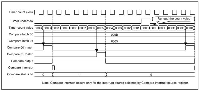
Fig. 45 Output compare mode (general waveform)
