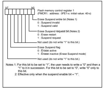
Fig. 99 Structure of flash memory control register 1
