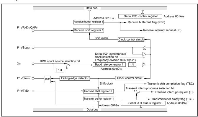
Fig. 55 Block diagram of clock synchronous serial I/O1
