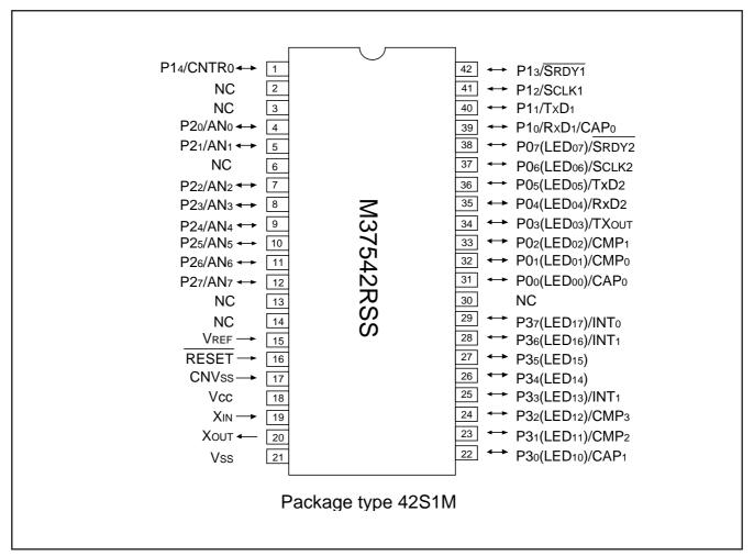
Fig. 5 Pin configuration (Package type: 42S1M)
