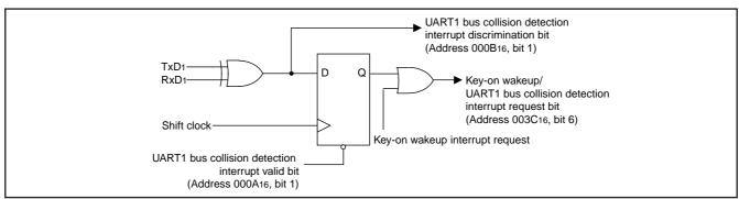
Fig. 61 Block diagram of bus collision detection interrupt circuit
