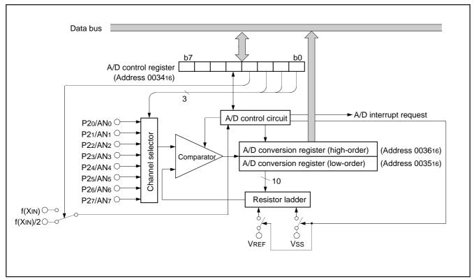
Fig. 70 Block diagram of A/D converter
