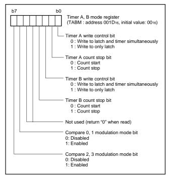
Fig. 32 Structure of timer A, B mode register
