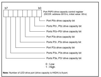
Fig. 17 Structure of port P0P3 drive capacity control register
