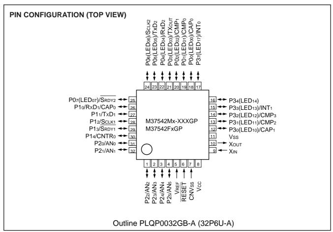
Fig. 1 Pin configuration (Package type: PLQP0032GB-A)
