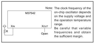
Fig. 76 Processing of XIN and XOUT pins at on-chip oscillator operation
