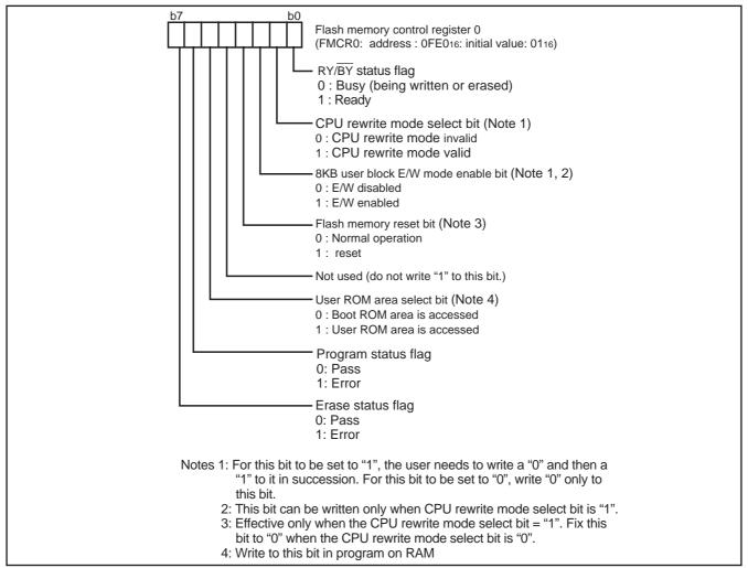
Fig. 98 Structure of flash memory control register 0
