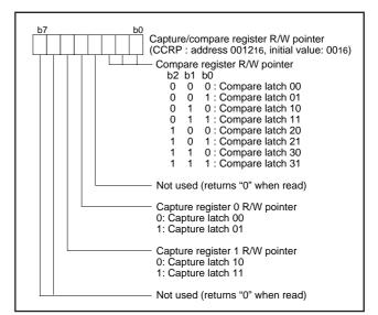
Fig. 35 Structure of capture/compare register R/W pointer
