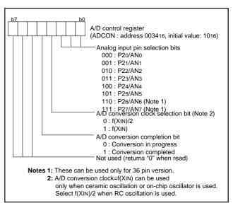
Fig. 68 Structure of A/D control register
