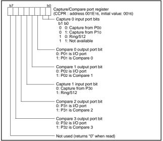
Fig. 37 Structure of capture/compare port register
