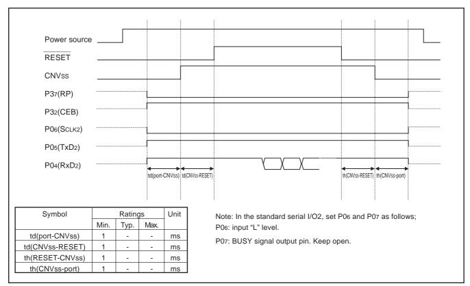
Fig. 116 Timing diagram in standard serial I/O mode 2
