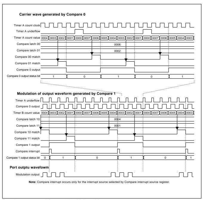
Fig. 47 Output compare mode (compare 0, 1 modulation mode)
