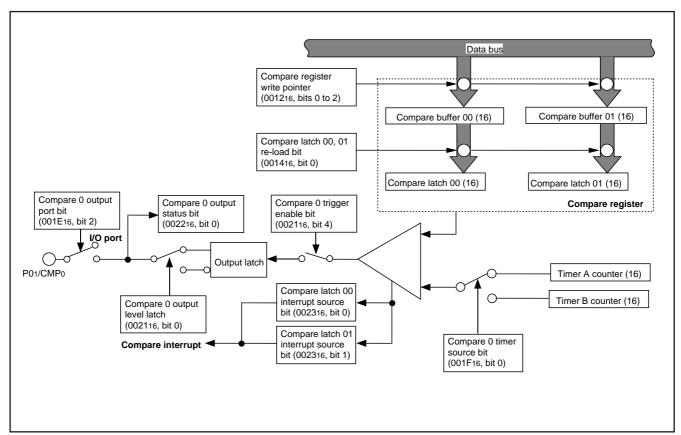
Fig. 43 Block diagram of compare channel 0
