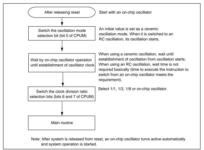
Fig. 14 Switching method of CPU mode register
