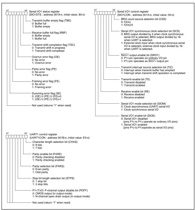
Fig. 59 Structure of serial I/O1-related registers
