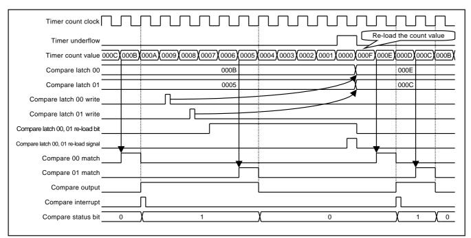
Fig. 46 Output compare mode (compare register write timing)
