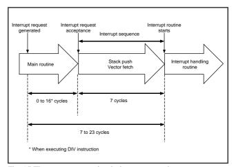
Fig. 25 Time up to execution in interrupt routine
