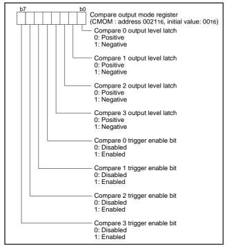
Fig. 39 Structure of compare output mode register
