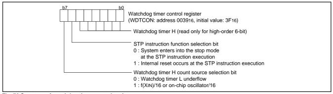
Fig. 72 Structure of watchdog timer control register
