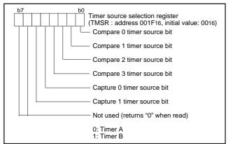
Fig. 38 Structure of timer source selection register
