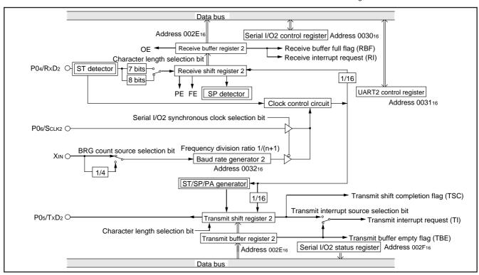
Fig. 65 Block diagram of UART serial I/O2
