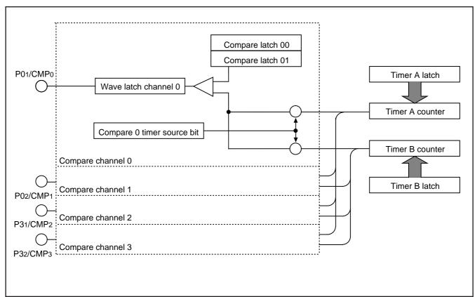
Fig. 42 Block diagram of output compare
