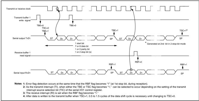
Fig. 58 Operation of UART serial I/O1 function
