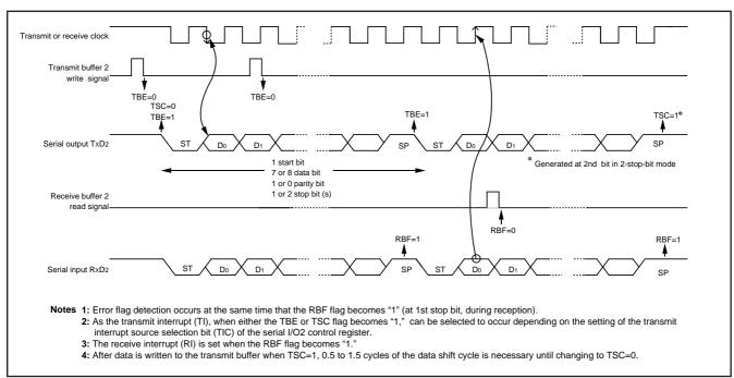
Fig. 66 Operation of UART serial I/O2 function
