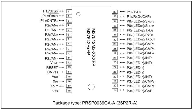
Fig. 2 Pin configuration (Package type: PRSP0036GA-A)
