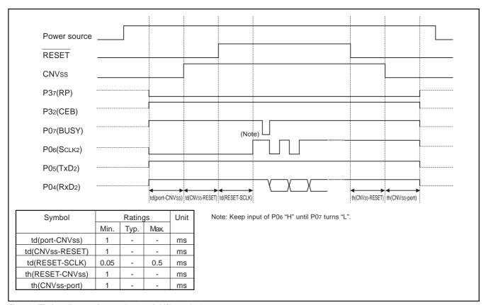
Fig. 111 Timing diagram in standard serial I/O mode 1
