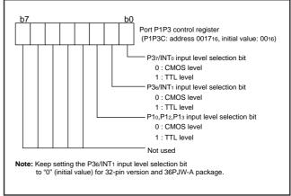
Fig. 19 Structure of port P1P3 control register
