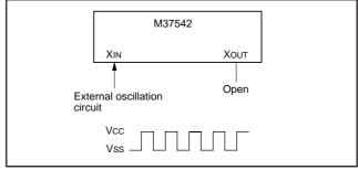
Fig. 79 External clock input circuit
