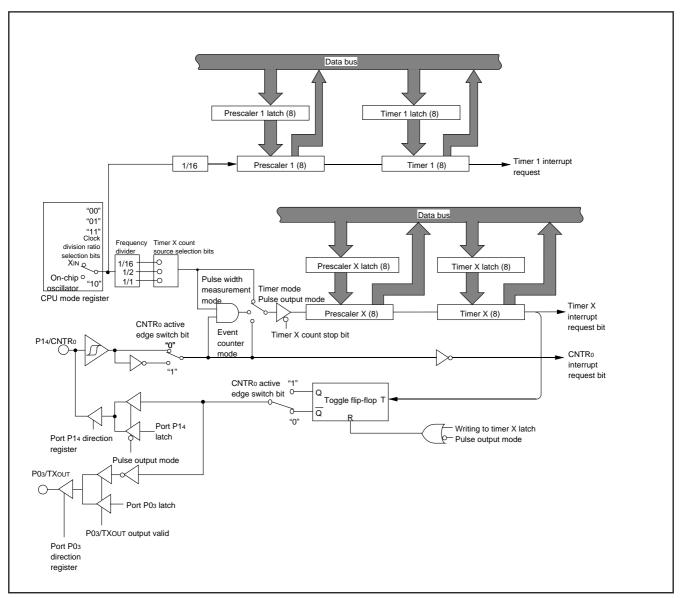
Fig. 31 Block diagram of timer 1 and timer X
