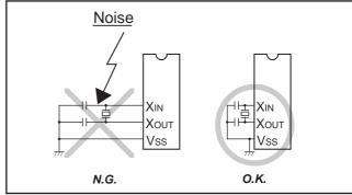
Fig. 89 Wiring for clock I/O pins
