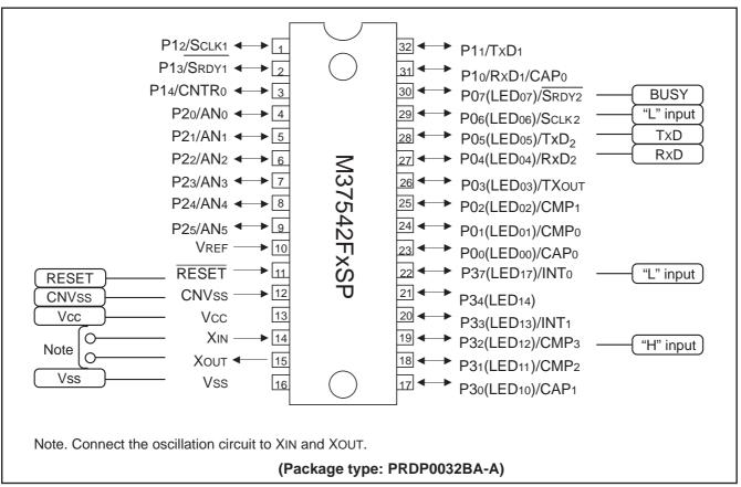
Fig. 114 Pin connection diagram in standard serial I/O mode 2 (PRDP0032BA-A package)
