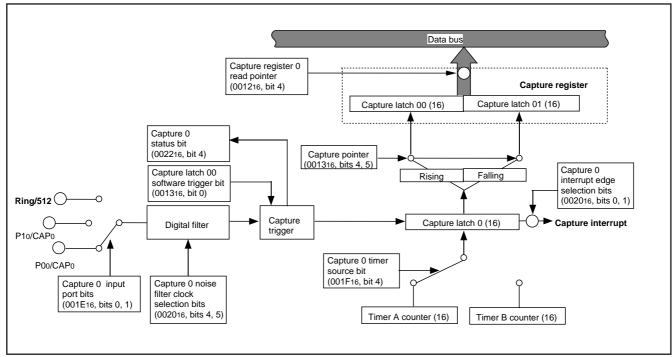
Fig. 52 Block diagram of capture channel 0
