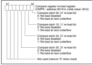
Fig. 36 Structure of compare register re-load register
