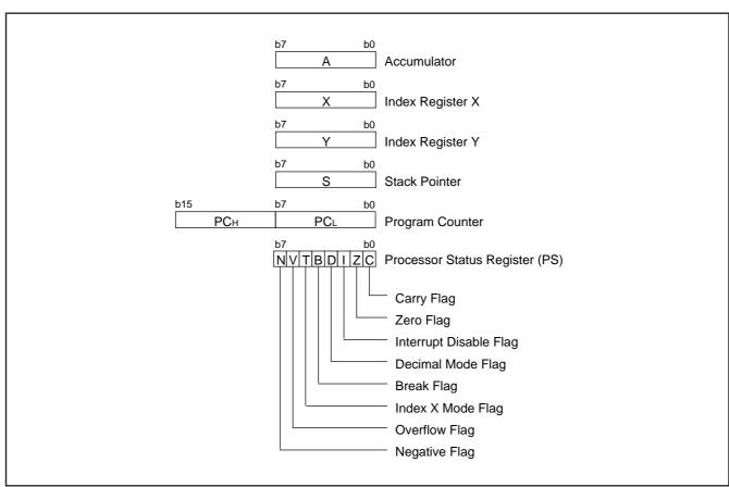
Fig. 11 740 Family CPU register structure
