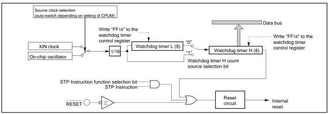
Fig. 71 Block diagram of watchdog timer
