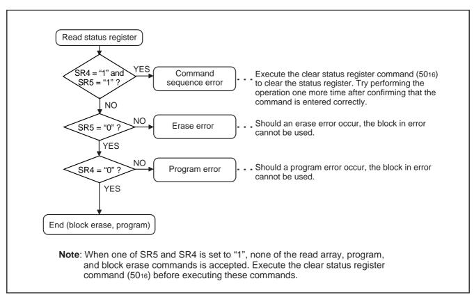
Fig. 104 Full status check flowchart and remedial procedure for errors
