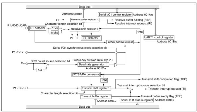
Fig. 57 Block diagram of UART serial I/O1
