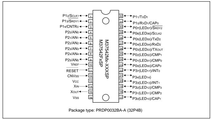
Fig. 3 Pin configuration (Package type: PRDP0032BA-A)
