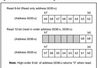
Fig. 69 Structure of A/D conversion register
