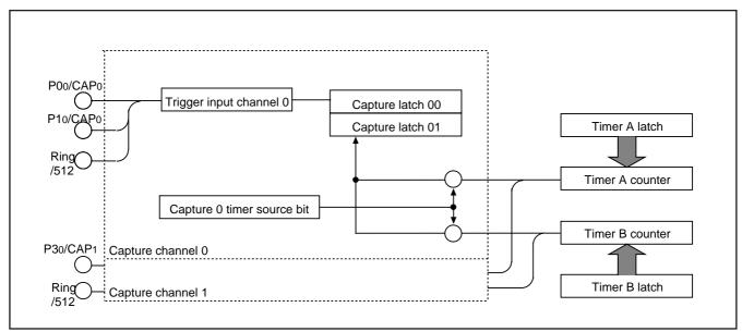
Fig. 51 Block diagram of input capture
