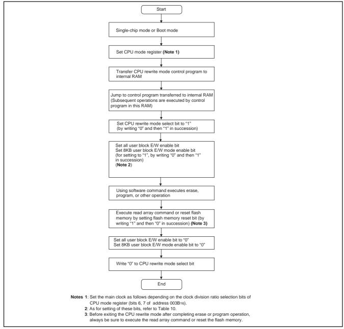
Fig. 101 CPU rewrite mode set/release flowchart
