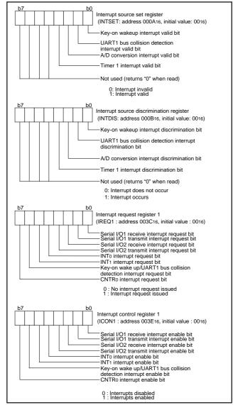
Fig. 60 Bus collision detection circuit related registers
