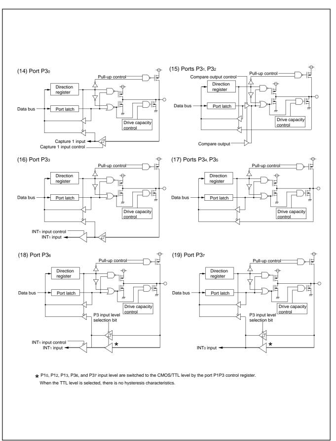
Fig. 22 Block diagram of ports (3)
