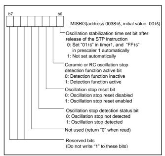
Fig. 85 Structure of MISRG
