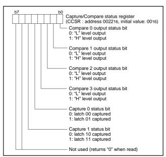
Fig. 40 Structure of capture/compare status register
