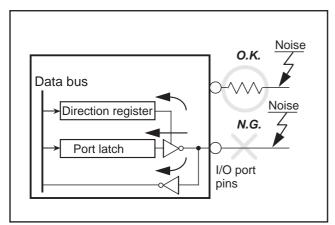
Fig. 95 Setup for I/O ports
