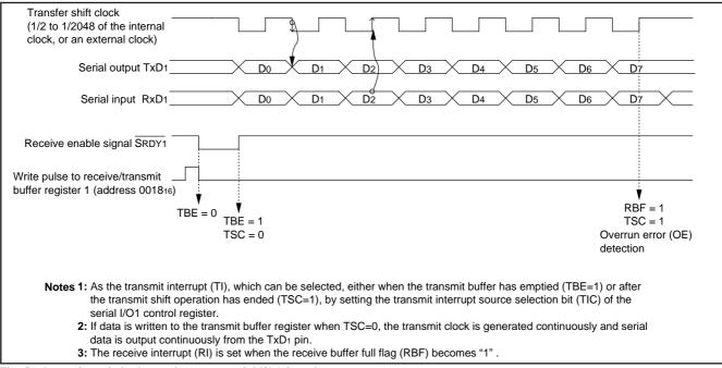
Fig. 56 Operation of clock synchronous serial I/O1 function
