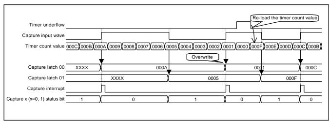
Fig. 53 Capture interrupt edge selection = "rising edge"
