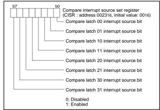
Fig. 41 Structure of compare interrupt source register
