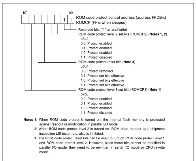
Fig. 105 Structure of ROM code protect control address
