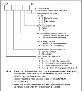
Fig. 13 Structure of CPU mode register
