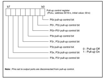
Fig. 18 Structure of pull-up control register
