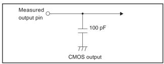
Switching characteristics measurement circuit diagram
