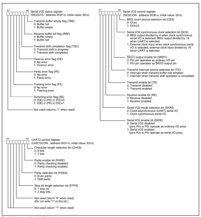
Fig. 67 Structure of serial I/O2-related registers
