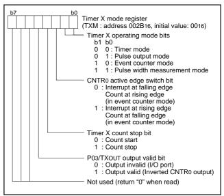
Fig. 29 Structure of timer X mode register
