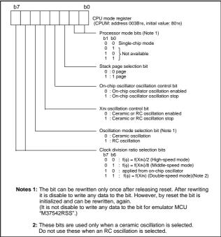
Fig. 80 Structure of CPU mode register
