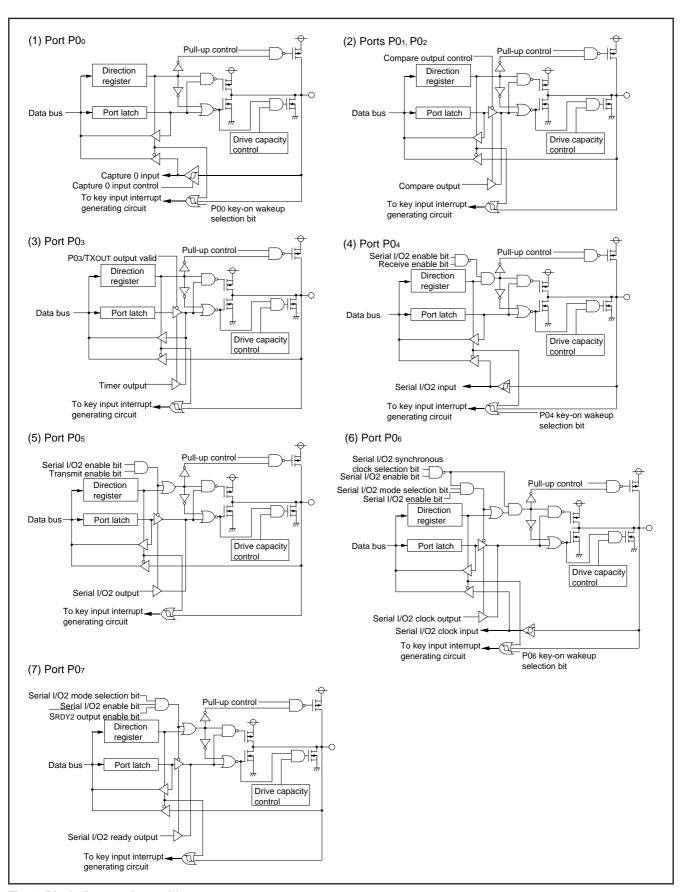
Fig. 20 Block diagram of ports (1)
