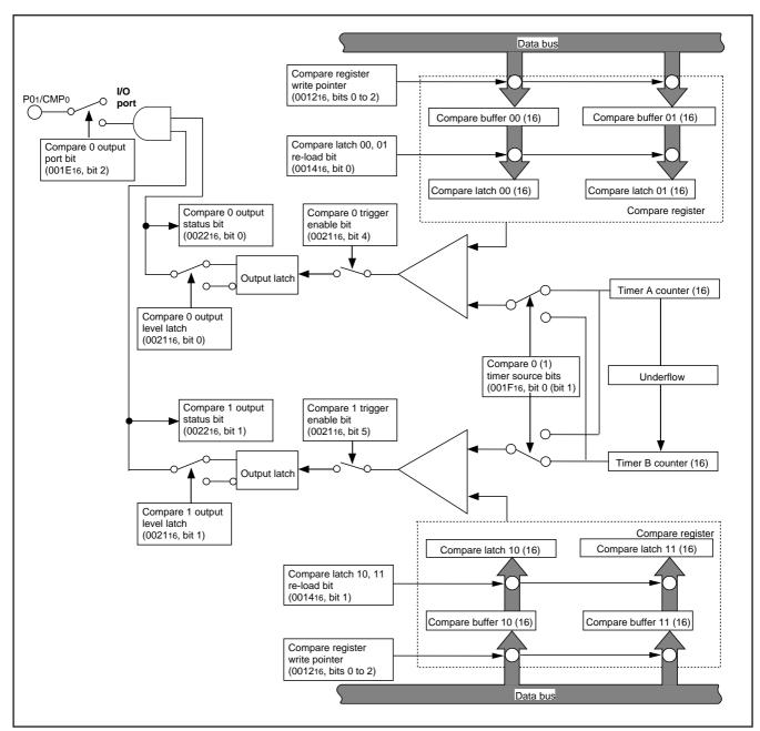
Fig. 44 Block diagram at modulation mode
