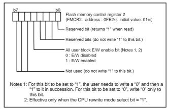
Fig. 100 Structure of flash memory control register 2
