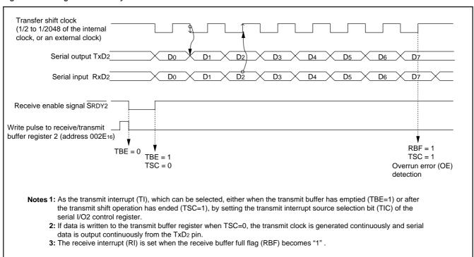
Fig. 64 Operation of clock synchronous serial I/O2 function
