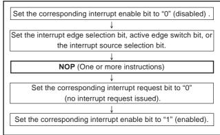
Fig. 4 Sequence of changing relevant register
