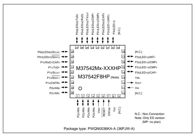
Fig. 4 Pin configuration (Package type: PWQN0036KA-A)
