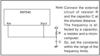
Fig. 78 External circuit of RC oscillation
