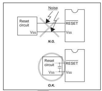
Fig. 88 Wiring for the  $\overline{\text{RESET}}$  pin
