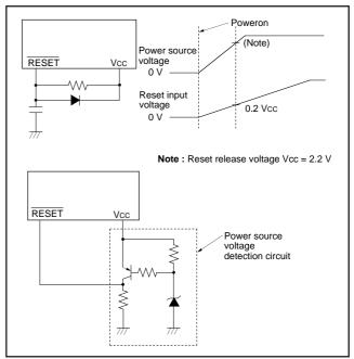
Fig. 73 Example of reset circuit
