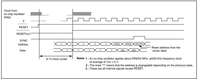
Fig. 74 Timing diagram at reset
