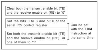
Fig. 6 Sequence of setting serial I/Oi control register again
