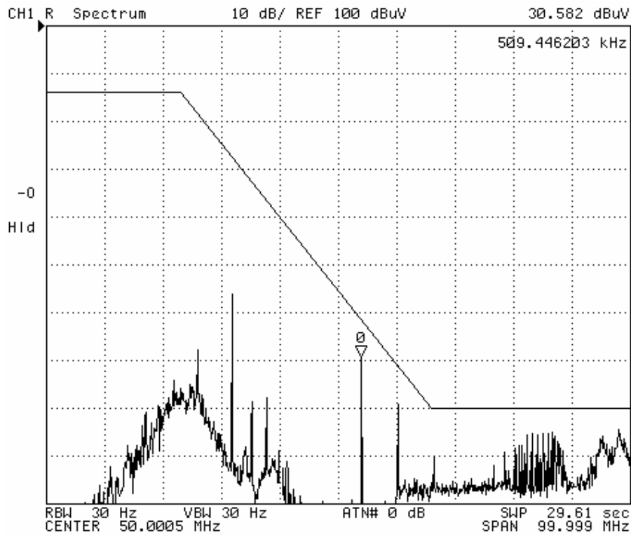
Fig 2. Typical Conducted Emissions, Positive Lead
