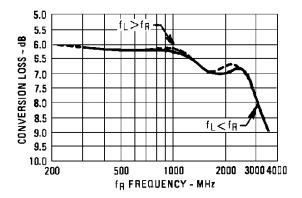
Conversion Loss vs. Input Frequency: Conversion loss of the mixer when used in an SSB system. Data plotted for a  $f_{\parallel}$  of 100 MHz with  $f_{\parallel}$  at +10 dBm.
