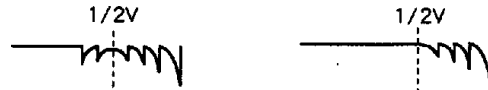
When pin ① is open When 35mV is applied to pin ①
