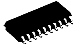
Outline 20P2N-A(AFP) 1.27mm pitch 300mil SOP (5.3mm x 12.6mm x 1.8mm)
