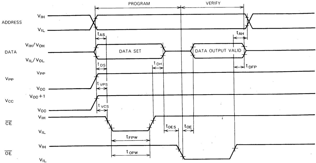
Test conditions for A.C. characteristics
