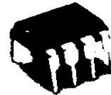
Outline 8P4 (P) 2.54mm pitch 300mil DIP (6.3mmx8.9mmx3.3mm)
