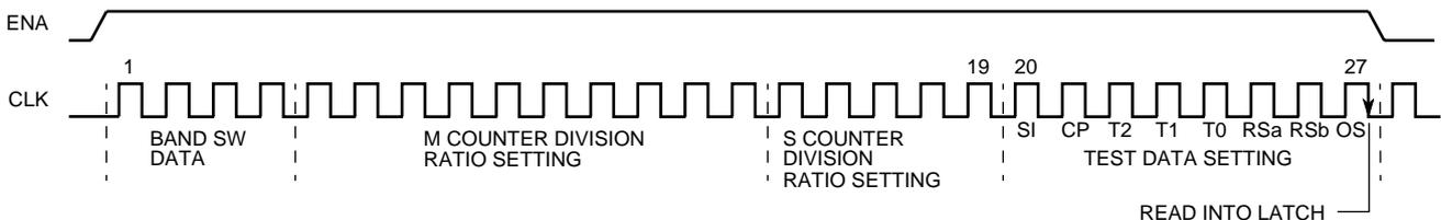
**SERIAL INPUT PLL FREQUENCY SYNTHESIZER FOR TV/VCR**
