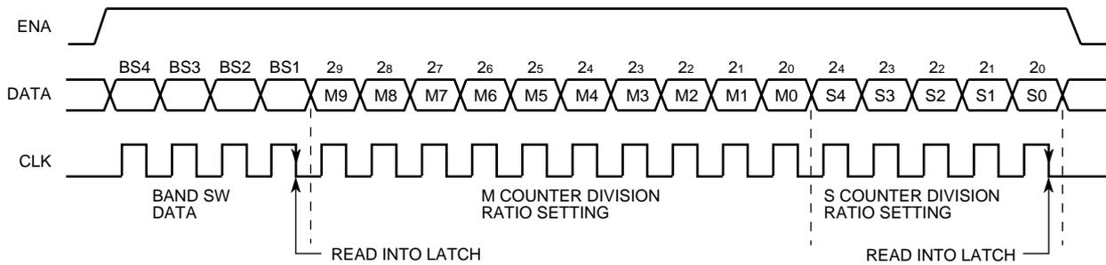
**HOW TO SET THE DIVIDING RATIO OF THE PROGRAMMABLE DIVIDER**
