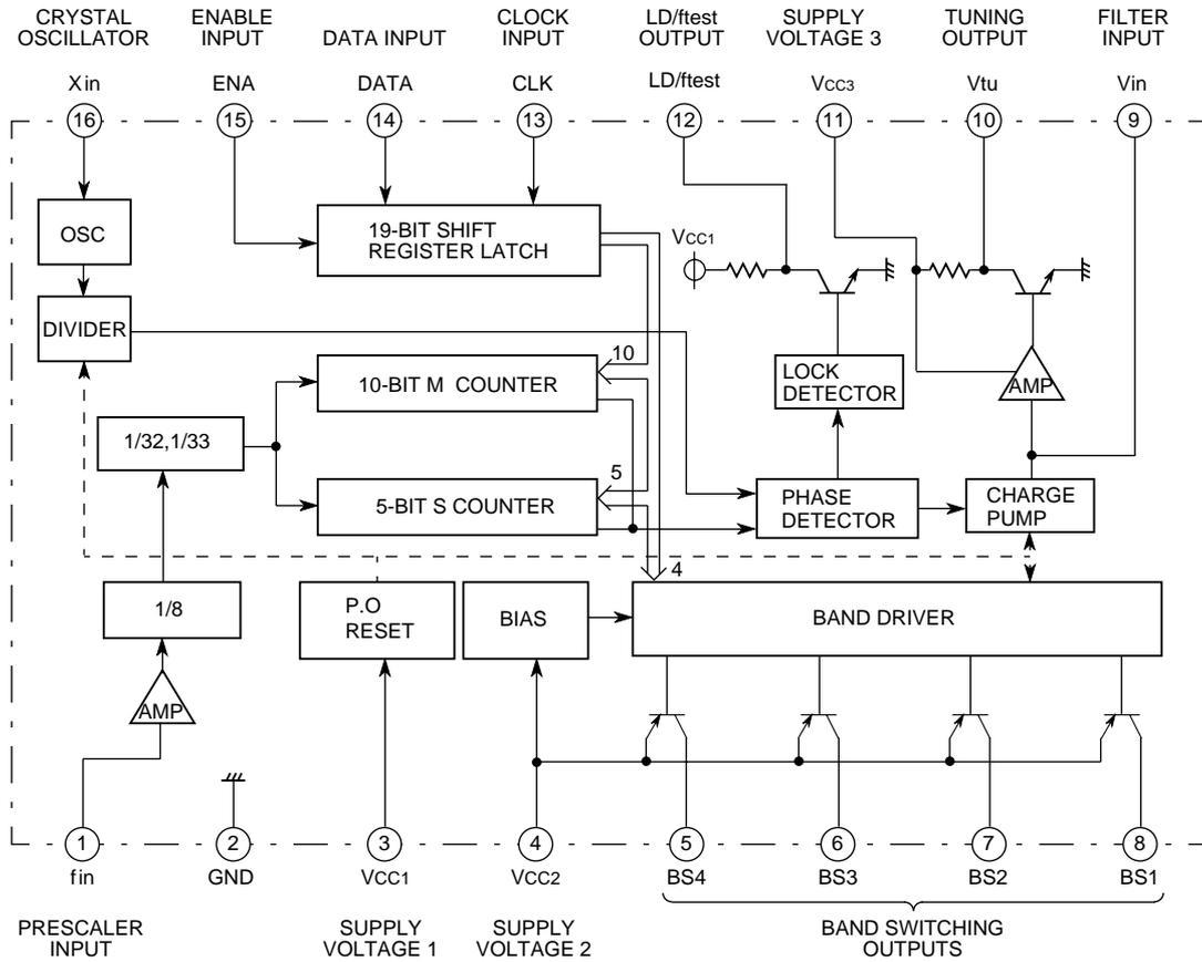
**SERIAL INPUT PLL FREQUENCY SYNTHESIZER FOR TV/VCR**
