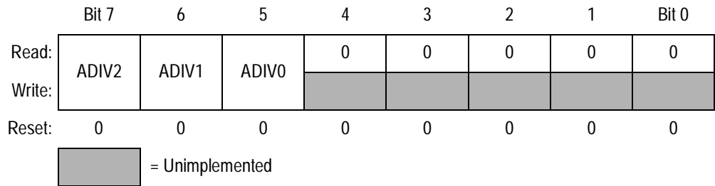
Figure 11-5. ADC Input Clock Register (ADICLK)
