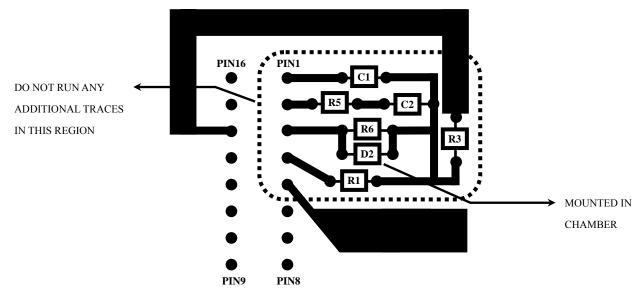
Notes : Illustration is bottom view of layout using a Dip. Top view for SOIC layout is mirror image. Optional potentiometer R2 is not illustrated drawing is not to scale. Leads on D2, R6, R1, and R3 and their associated traces must be kept as short as possible. This practice minimizes noise pick-up. Pin 3 must be decoupled from all other traces.
