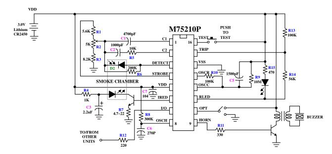
\* C2 and R7 are used for coarse sensitivity adjustment. Typical values are shown.
