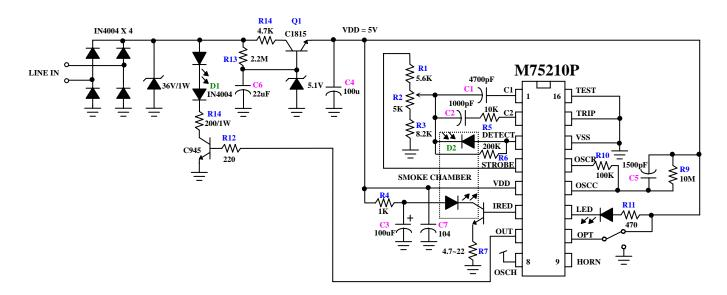
\* C2 and R7 are used for coarse sensitivity adjustment. Typical values are shown.
