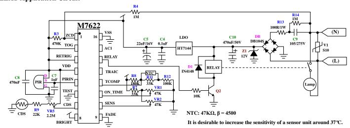
$\begin{aligned} \textbf{RETRIG} &= \textbf{VDD} : \textbf{Retrigger} \\ &= \textbf{VSS} : \textbf{Non-Retrigger} \end{aligned}$
