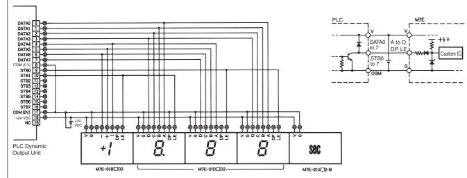
2. Connected to C200-OD215 Transistor Output Unit
