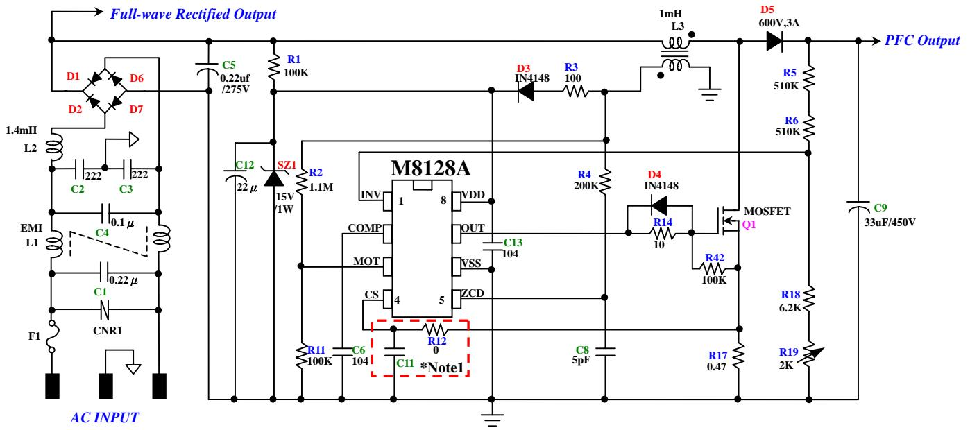
\* Note1 : Compensation network between CS pin and VSS
