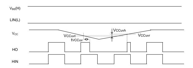
If  $V_{BS}$  Supply voltage drops below UV trip voltage ( $V_{BSuvt} = V_{BSuvr} - V_{BSuvh}$ ) for  $V_{BS}$  supply UV filter time, output signal HO becomes "L". As soon as  $V_{BS}$  supply voltage rises over UV reset voltage, output signal HO becomes "H" at following "H" edge of input signal.
