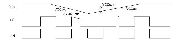
If  $V_{CC}$  Supply voltage drops below UV trip voltage ( $V_{CCuvt} = V_{CCuvr} - V_{CCuvh}$ ) for  $V_{CC}$  supply UV filter time, output signal HO becomes "L". As soon as  $V_{CC}$  supply voltage rises over UV reset voltage, output signal HO becomes "H" it input signal is "H".
