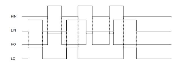
Note1 :The minimum input pulse width at HIN/LIN should be to more than 500ns (because of HIN/LIN input noise filter circuit). Note2 :Delay times between input and output signals are not shown in the figure above.
