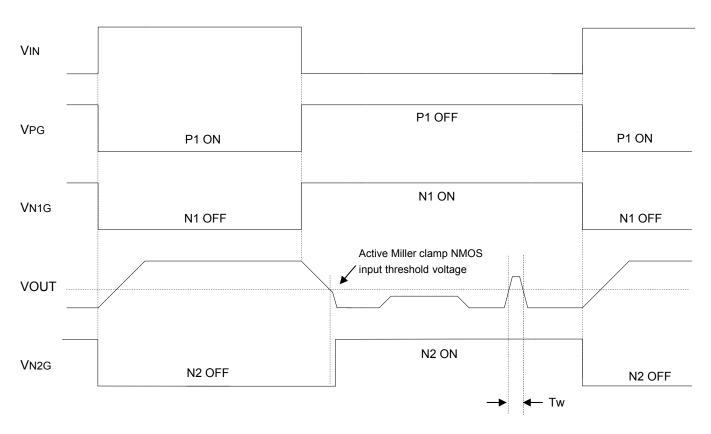
Active Miller effect clamp NMOS  $\,$  keeps turn-on if  $T_W$  does not exceed active Miller clamp NMOS filter time
