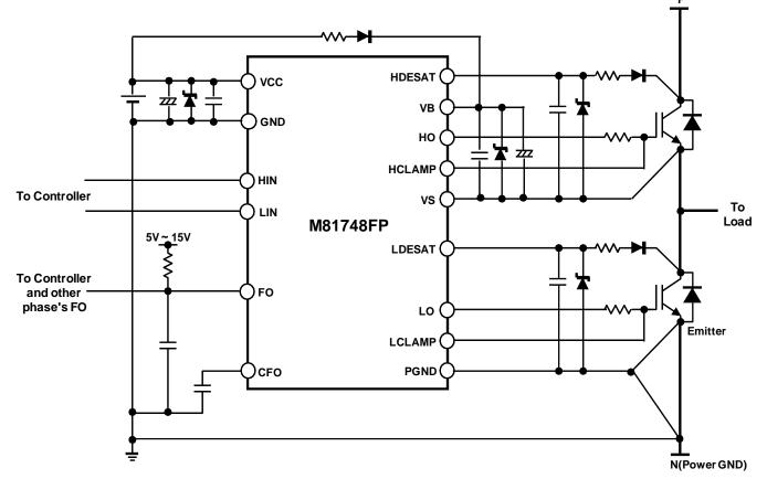
Note: If HVIC is working in high noise environment, it is recommended to connect a 1nF ceramic capacitor to FO pin. It is recommended to connect PGND pin to Emitter and Power GND(N). If PGND pin is not connected to Power GND(N), please pay attention to a noise between PGND pin and Power GND(N).
