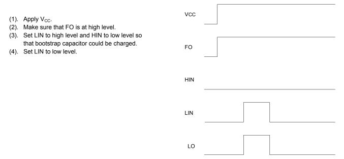
Note : If two power supply are used for supplying V<sub>CC</sub> and V<sub>BS</sub> individually, it is recommended to set V<sub>CC</sub> first and then set V<sub>BS</sub>.
