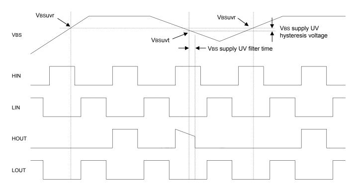
Note1 :Delay times between input and output signals are not shown in the figure above.
