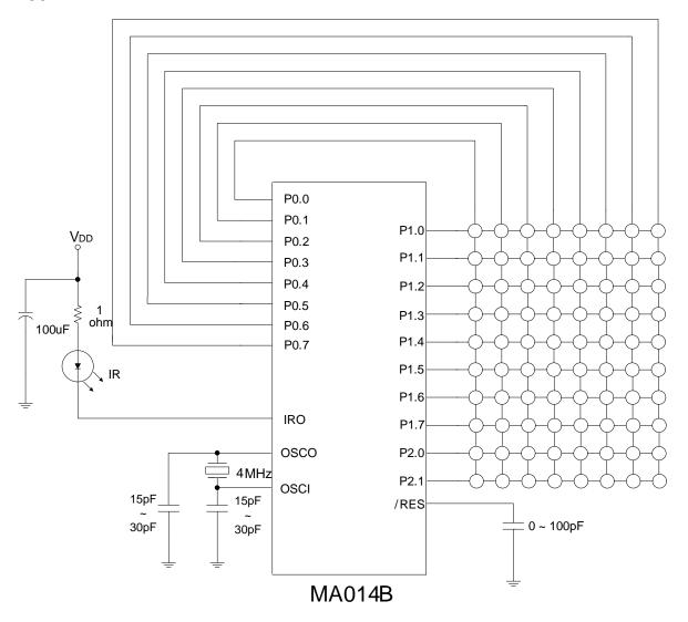
Note: No capacitor or below 100pF capacitor is strongly recommended to connected on /RES pin.
