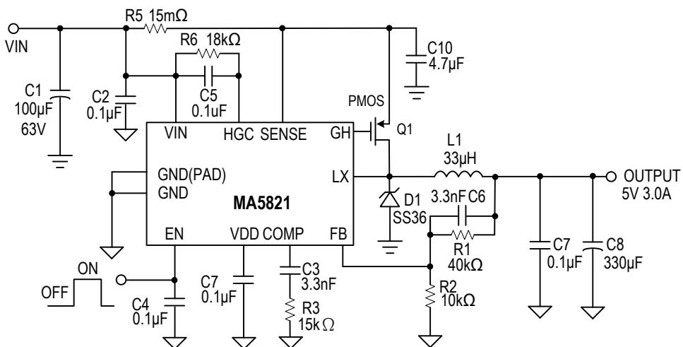
$$V_{OUT} = V_{FB} \times (1 + R1/R2), \quad V_{FB} = 1.0V, \quad R2 \text{ suggest } 1K \sim 30K\Omega.$$
