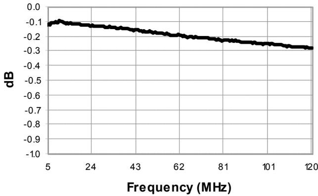
Insertion Loss 2 (Pin5 - Pin3)
