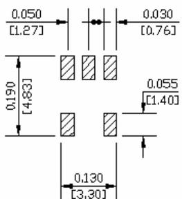
Dimensions are inches [millimeters]  $\pm 0.015$  [0.38] unless otherwise specified.
