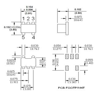
Dimensions are inches (millimeters) ±0.015 (0.38) unless otherwise specified. Drawing not to scale
