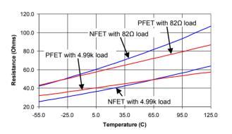
6. Output resistance were measured under the condition of  $V_{CC}$  = +5.0 V,  $V_{OPT}$  = +5.0 V, and  $V_{EE}$  = -5.0 V, with load resistors from outputs to ground.
